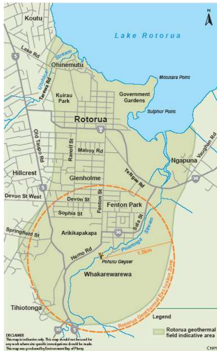
Figure 37: Extent of Rotorua Geothermal Field as defined by resistivity surveys. The map is taken from Gordon et al (2001).
