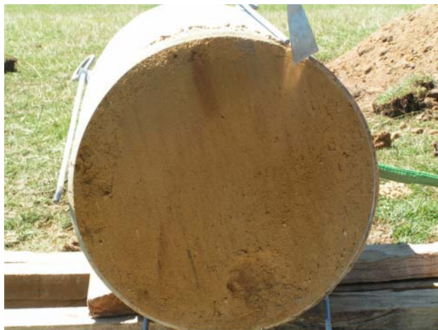
Figure 6.10 Cutting plate removed.
