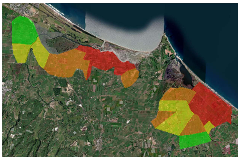
Figure 8 - Areas separated by line capacity. Green (3+MW), Yellow (2-3MW), Orange (1.5-2MW), Red (1-1.5MW), Grey (0-1MW)
