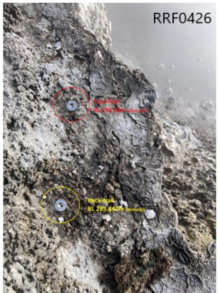
RRF0426 Unnamed feature current datum (front nail – red circle). Back-nail was installed and surveyed already for backup.
