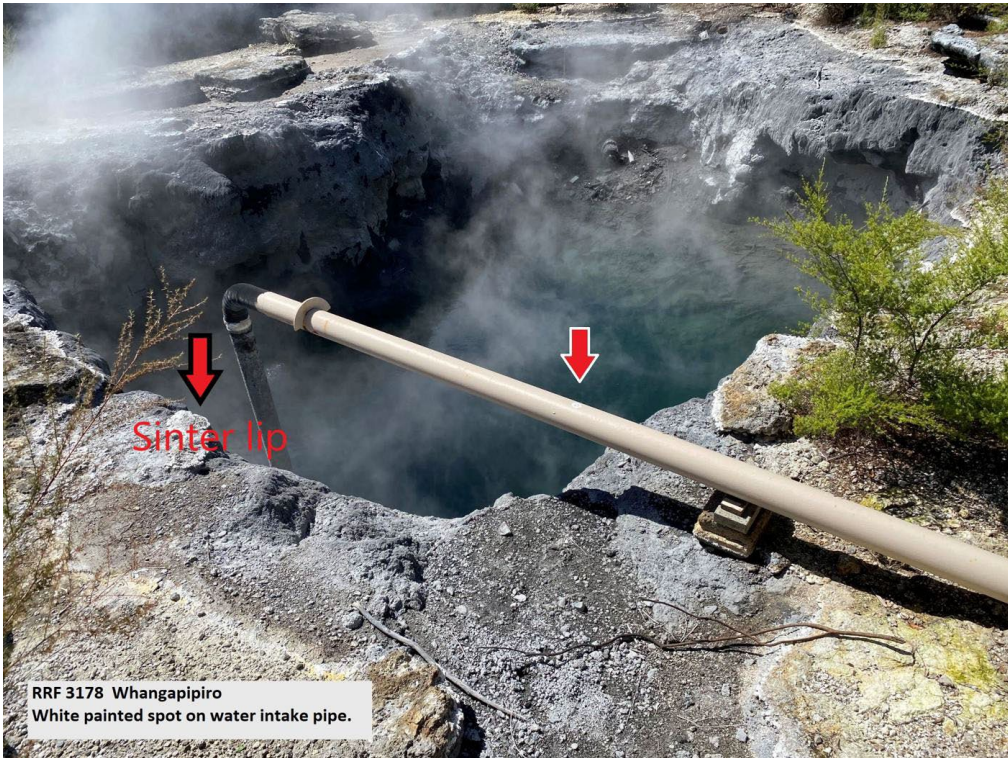
RRF3178 Whangapiro / Rachel Spring old datum (sinter lip) and new datum (top of pipe).
