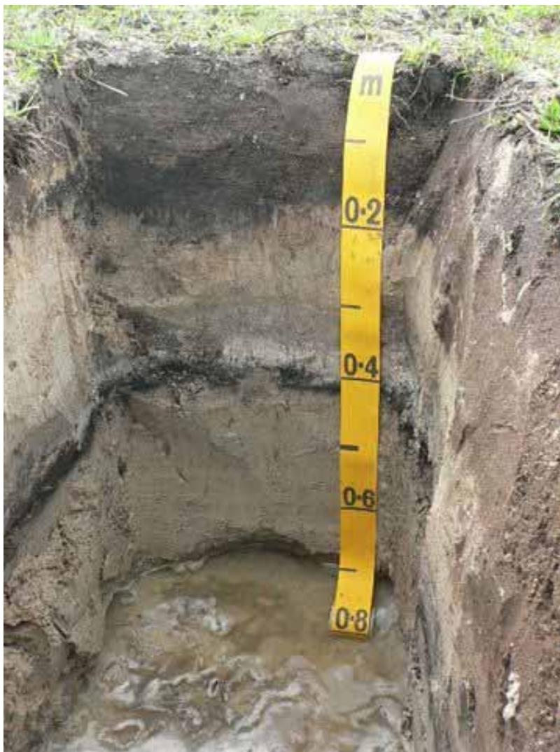
Awaiti sand (Note subsoil mottling and thin layer of Kaharoa Tephra at 40 cm depth)
