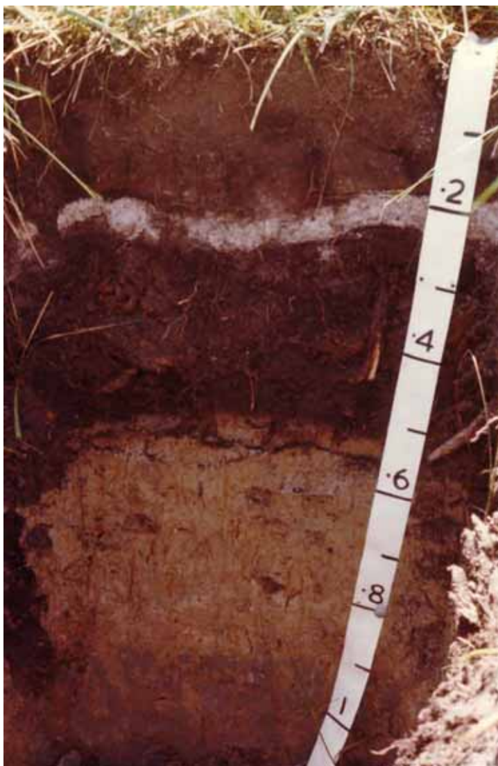
Paerata peaty silt loam (Note Kaharoa Tephra at 20 cm depth, scale in m)
