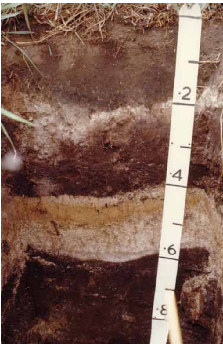
Matao peaty silt loam (Note Kaharoa Tephra at 20 cm and Taupō Tephra at 40 to 60 cm depth)
