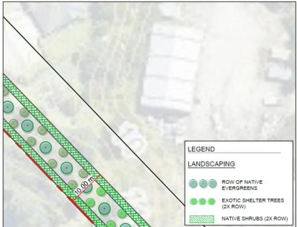
**Figure 3:** Zoomed-in excerpt of MPAD Drawing 'Landscape Plan – Permitted Works – Boundary Landscaping', showing the 5x rows of planting to perimeter locations, with legend inset. This detail of landscaping was prepared by the applicant's landscape architect and confirmed consistent with the landscaping requirement of Te Puna Business Park Structure Plan so as to satisfy Rule 12.4.16.3.b.
