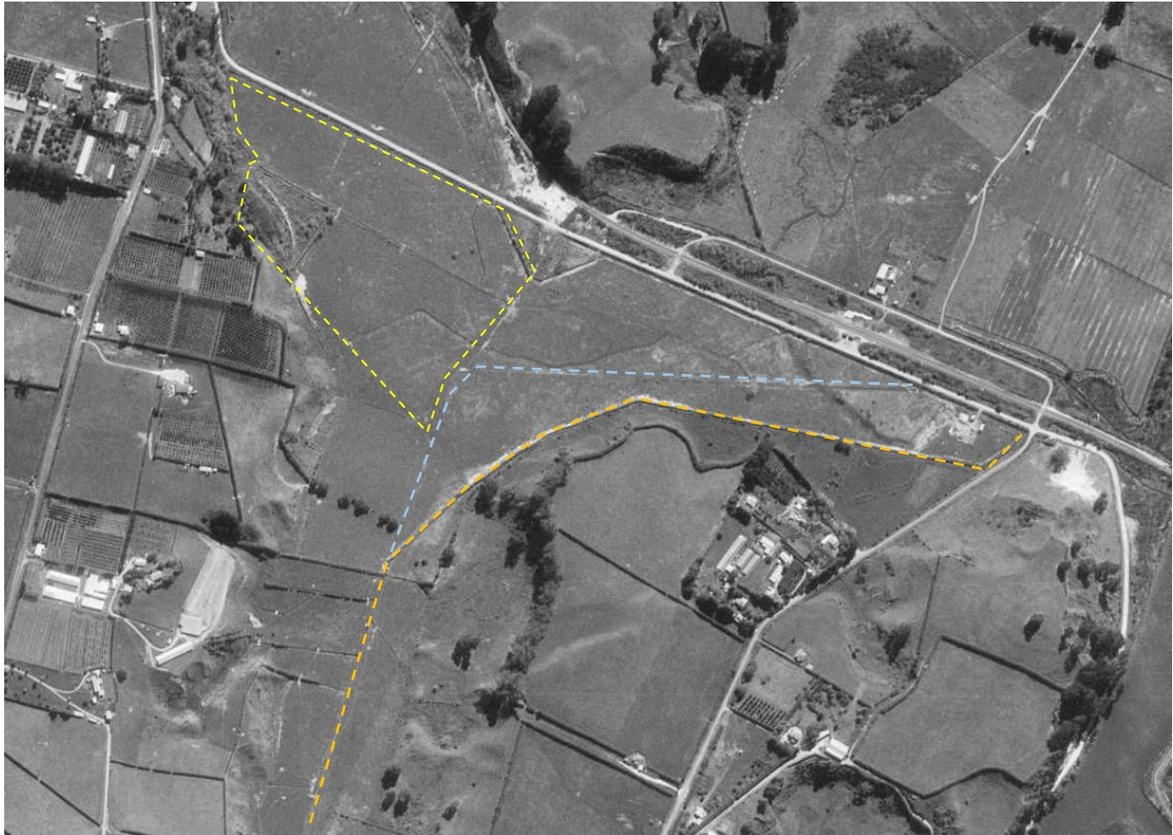
**Figure 7. Aerial Photo taken in 1974 showing the altered main drain alignment (orange broken line) and the abandoned drain (Light blue broken line). NZAM Neg.SN3731 H5.**
