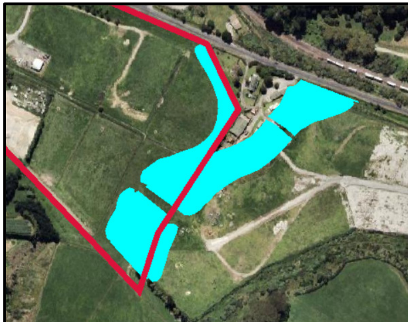
Figure 3.3 – Structure Plan overland flow path designation
