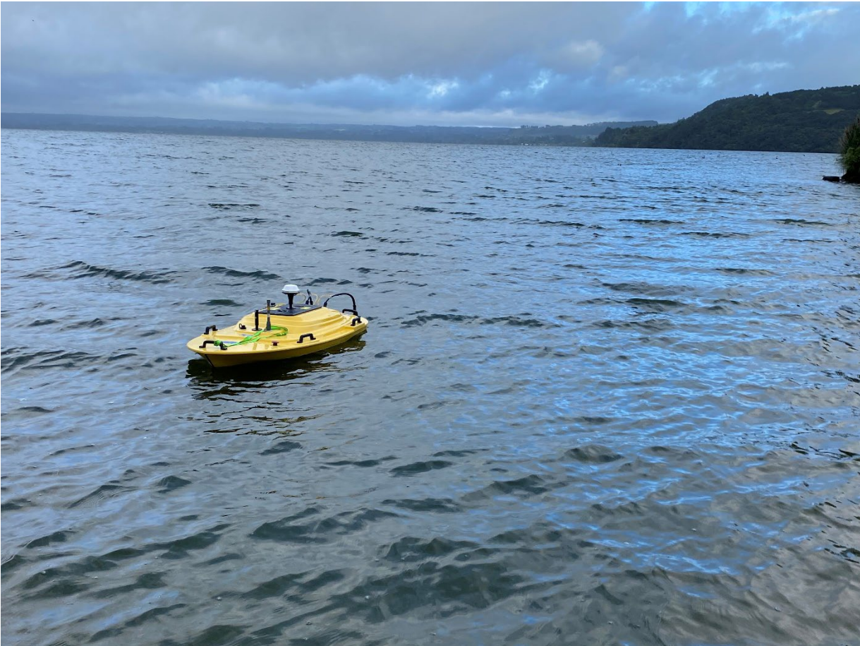
Figure 1 Calculating the Ōhau Channel Flow Rate with the 'Q-Boat' 5 March 2024
