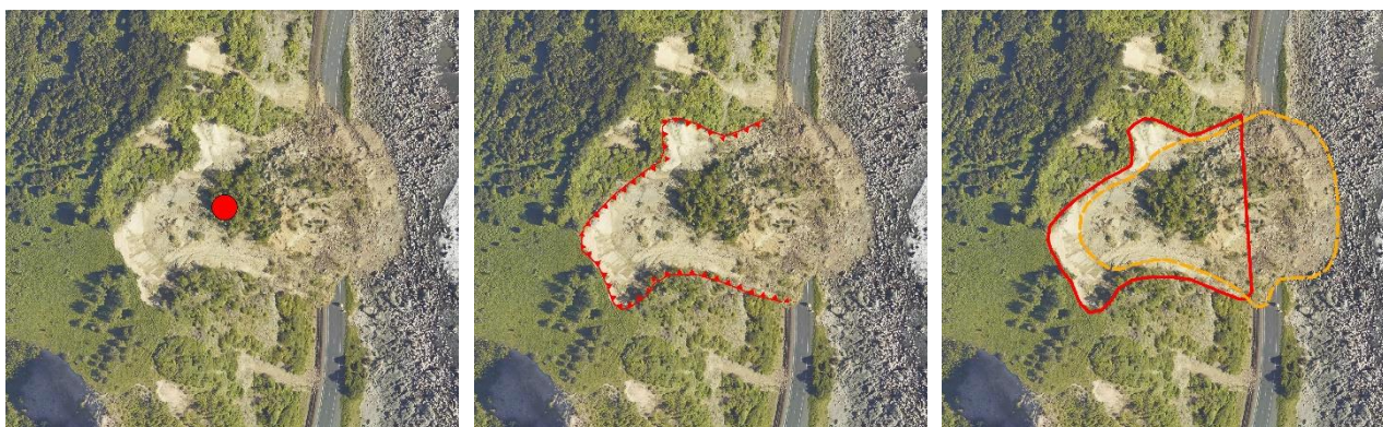
Figure 8 Examples of how landslides are depicted in GIS (A) Point within the landslide body; (B) Line around the head scarp of the landslide; (C) Polygons delineating the failure zone (red solid line) and the debris runout zone (orange dashed line)
