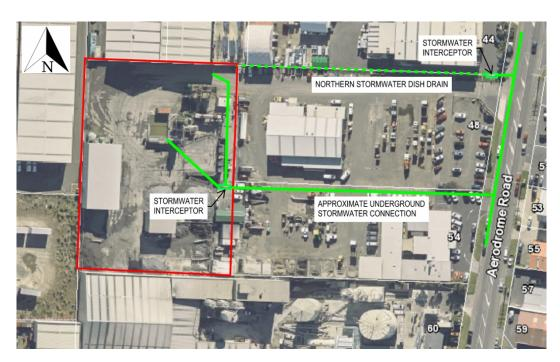
Figure 1: Existing stormwater network at 54 Aerodrome Road with Allied Asphalt site boundary in red.
