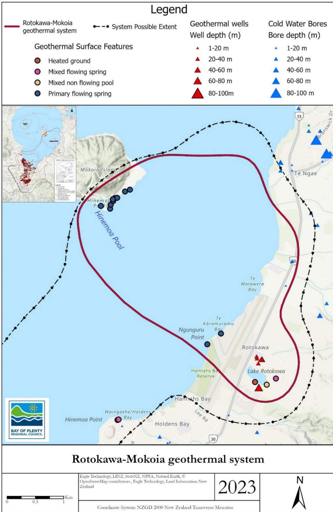
Figure 4: Rotokawa-Mokoia Geothermal System extent and a potential zone of hydrological connection with the Rotorua Geothermal System. Location and type of the geothermal surface features (dots). Location and depth category of the geothermal and cold wells (triangles). Surface feature data from GNS Science Geothermal Groundwater database (filtered).
