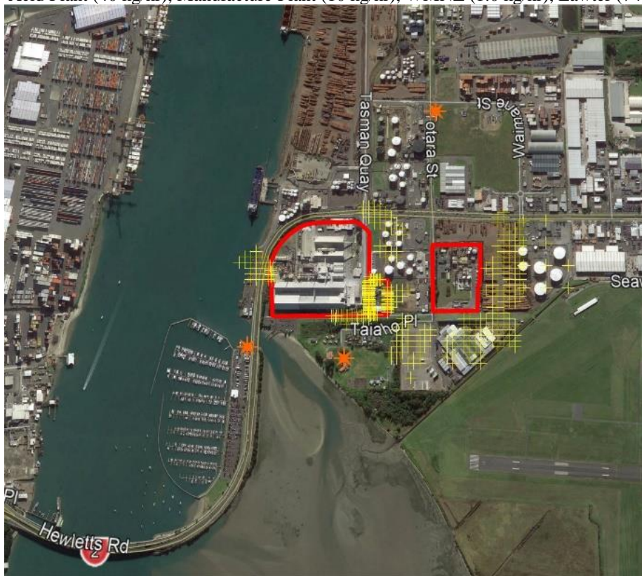
Figure 3-3. Locations showing the exceedances of the 24-hour modelled SO 2 concentrations ( \mu\text{g}/\text{m}^3 ) where Acid Plant (40 kg/hr), Manufacture Plant (10 kg/hr), WMNZ (1.0 kg/hr), Lawter (74 kg/hr).
