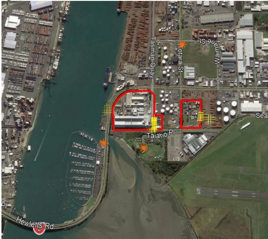
Figure 3-3. Locations showing the exceedances of the 24-hour modelled SO 2 concentrations ( \mu\text{g}/\text{m}^3 ) where Acid Plant (40 kg/hr), Manufacture Plant (10 kg/hr), WMNZ (1.0 kg/hr), Lawter (74 kg/hr).
