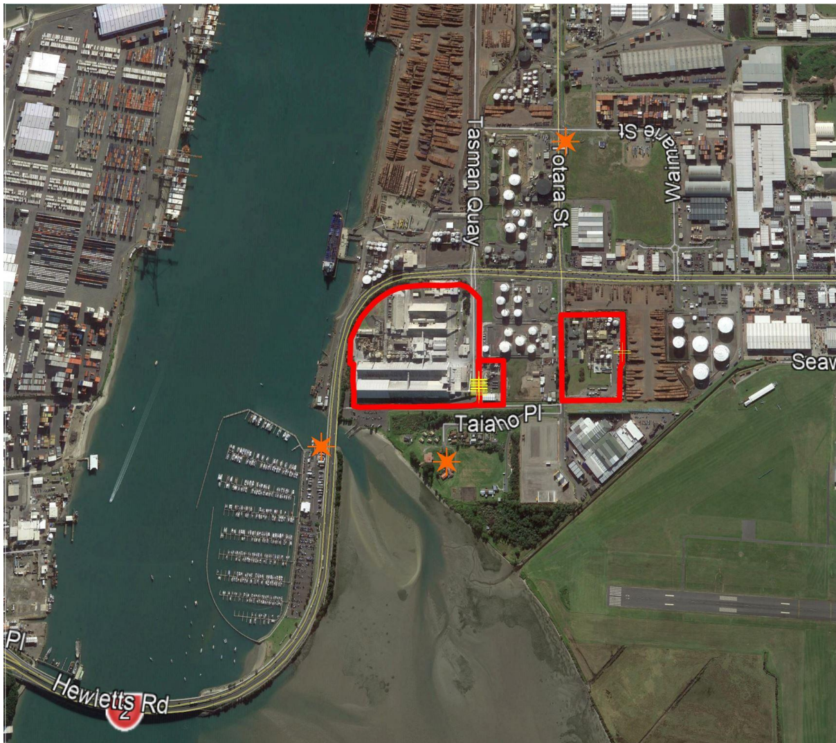
Figure 2-10. Scenario 4 – Locations showing the exceedances of the maximum 1-hour modelled SO 2 concentrations (µg/m 3 ) where Acid Plant (30 kg/hr), Manufacture Plant (5 kg/hr), WMNZ (0.8 kg/hr), Lawter (40 kg/hr).
