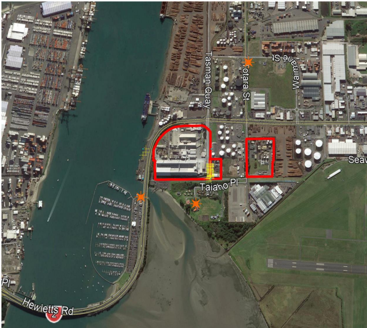
Figure 2-12. Scenario 4 – Locations showing the exceedances of the 24-hour modelled SO 2 concentrations ( \mu\text{g}/\text{m}^3 ) where Acid Plant (30 kg/hr), Manufacture Plant (5 kg/hr), WMNZ (0.8 kg/hr), Lawter (40 kg/hr).
