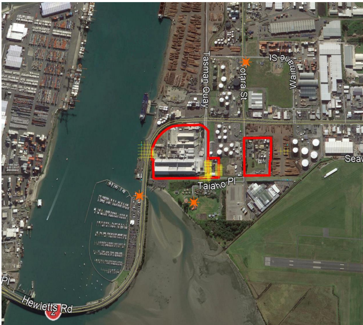
Figure 2-3. Scenario 1 – Locations showing the exceedances of the 24-hour modelled SO 2 concentrations (µg/m 3 ) where Acid Plant (40 kg/hr), Manufacture Plant (10 kg/hr), WMNZ (1 kg/hr), Lawter (58 kg/hr).
