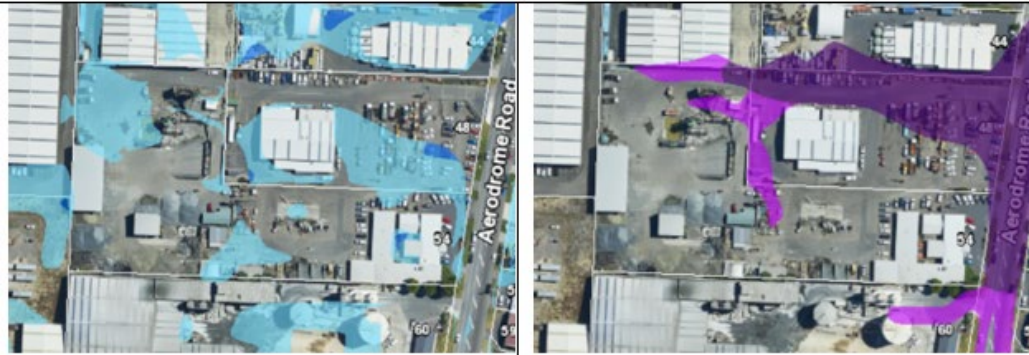
Figure 3 - Aerial view of the site showing Flood Prone Area overlay (blues), Minor Overland Flowpath (light purple) and Major Overland Flowpath (dark purple) (Source: AEE).
