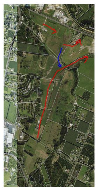
Our assessment of the direction of flow of water from the Container Co site is that it currently either flows through the Tinex site to the east via the culvert, or backs up behind the small culvert, flows south and then east to discharge to the stream (secondary flow path marked in GREEN), and that the only inflows are from the hills to the south and west, and a small amount of the catchment behind, extending as far back as Te Puna road;
