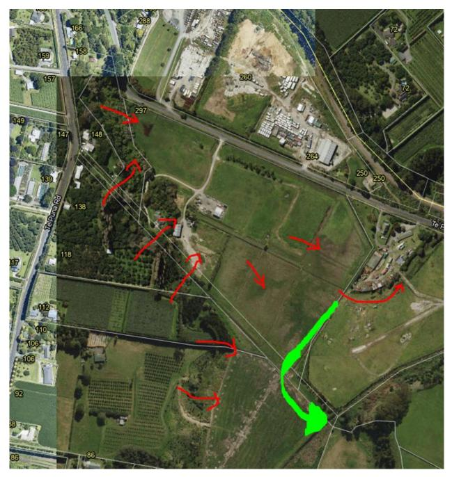
ContainerCo are only required to consider and mitigate the stormwater from their own operation, and that which flows directly through the site – not that from the wider catchment that the Container co site discharges to. We have calculated the stormwater flow rate for the current situation and that from the proposed development, and mitigated accordingly, as per the consent application, and the previously submitted stormwater spreadsheet.
