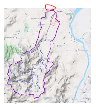
Even if there is some flow from the larger catchment into the ContainerCo Site, the bulk of the upstream flow passes by the ContainerCo site, flowing directly down the stream. There is under some circumstances a secondary flow path from the ContainerCo site (marked below in blue) when the area downstream of the ContainerCo site is flooded, or the capacity of the small culvert on the Tenix boundary is exceeded;
