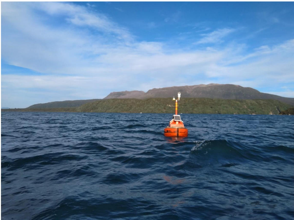
Figure 2 Monitoring buoy in Lake Tarawera, which supports high-frequency (15-min) meteorological and water quality measurements.
