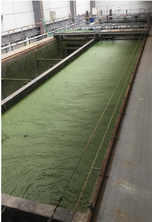
Figure 10 Example of harvesting and concentrating cyanobacteria (mostly Microcystis spp.) in water from Lake Taihu where concentrations are extremely high and the lake area is 2,390 km 2 . Photo: M. Burford.
