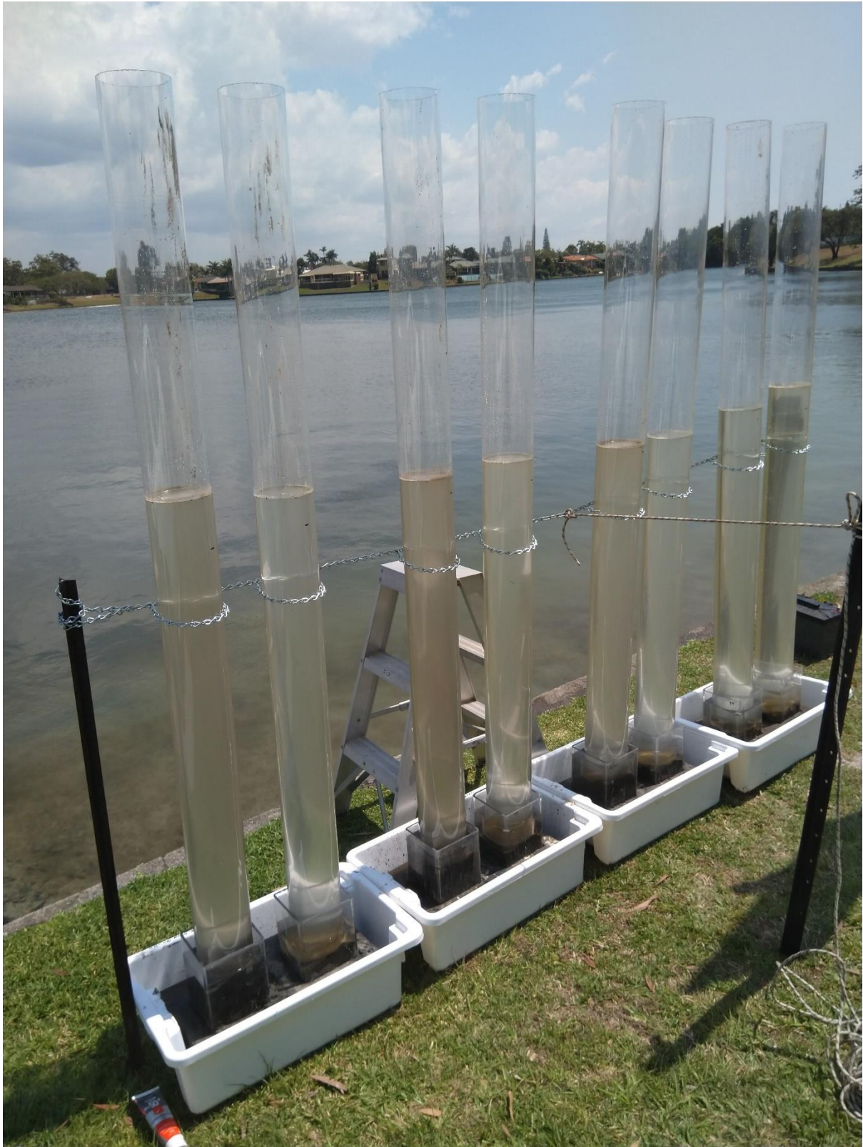
Figure 4 Small-scale experiments using controls and various concentrations of flocculants are essential to build a body of evidence on the efficacy of flocculants at different doses.
