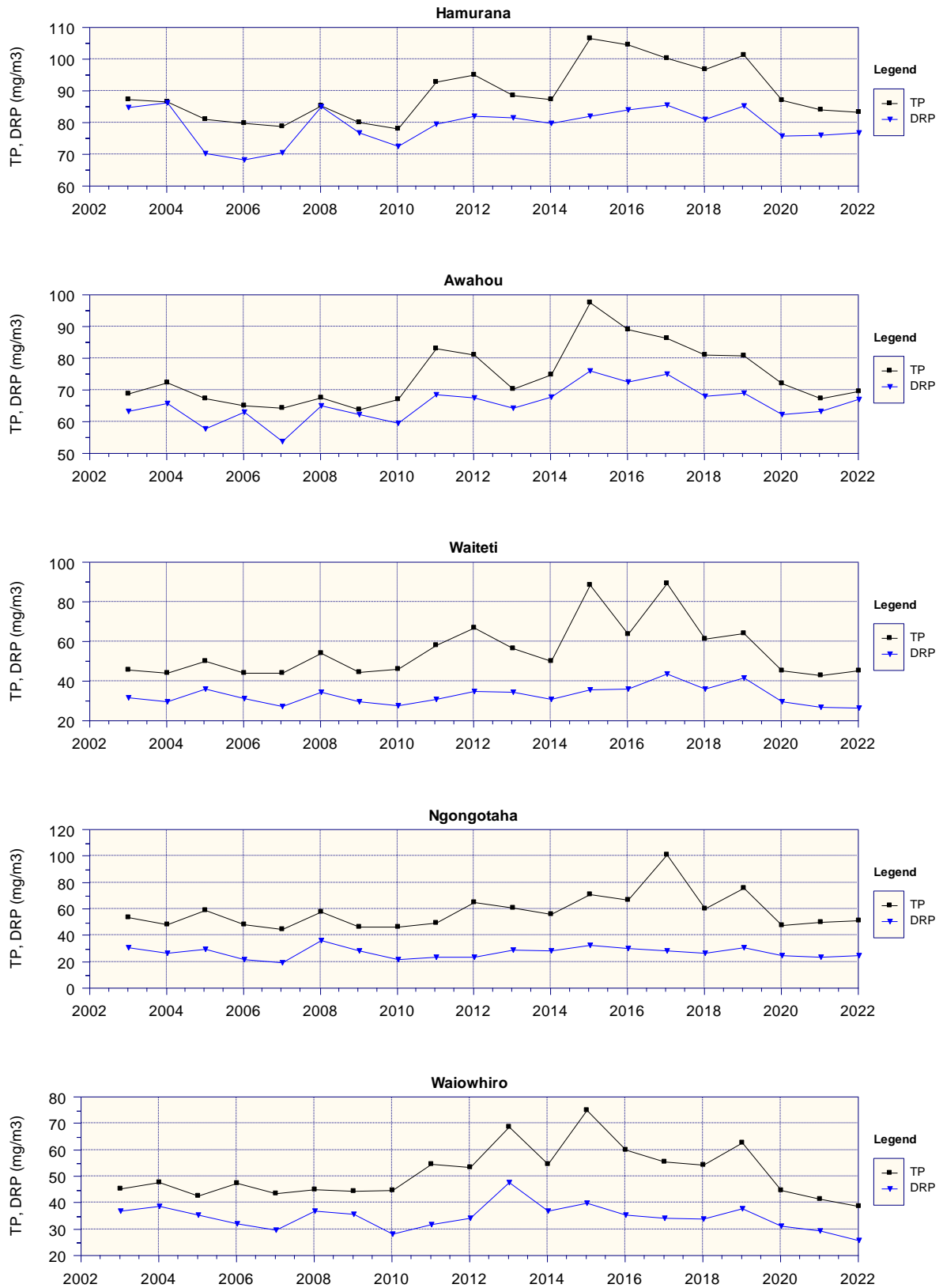
Figure 3.7 a: Annual average phosphorus concentrations in the main streams entering Lake Rotorua.
