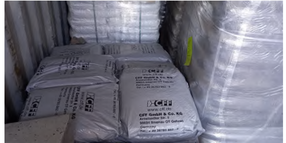
Photo 10: Bags of cellulose fibres used for asphalt production stored in shipping container located on the eastern site boundary beside the entrance.
