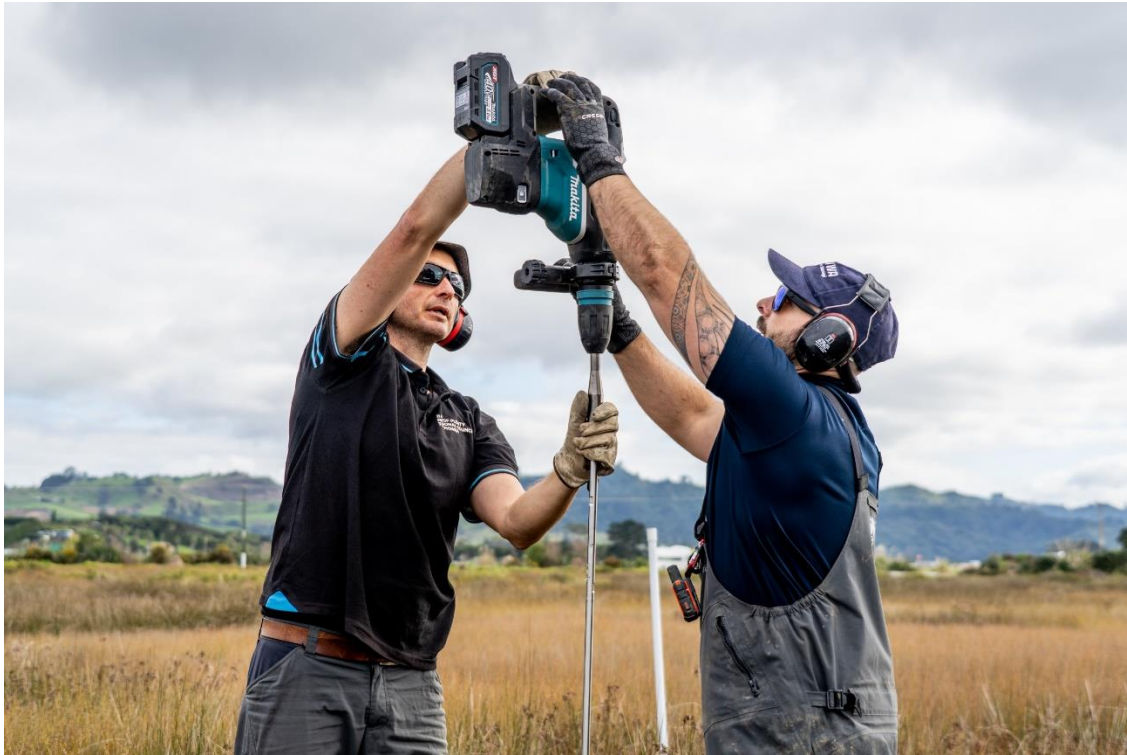
Figure 2-13: Battery Powered Hammer Drill used for driving SS rods into the sediment.
