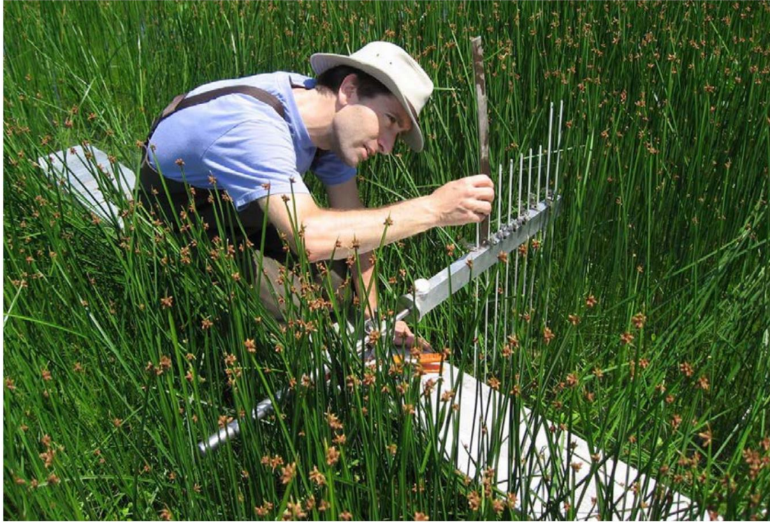
Figure 2-23: Reading the pin heights for SET instrument. Reproduced from US Geological Survey publication: The Surface Elevation Table and Marker Horizon Technique: A Protocol for Monitoring Wetland Elevation Dynamics. SOP-4, Figure 4.20.
