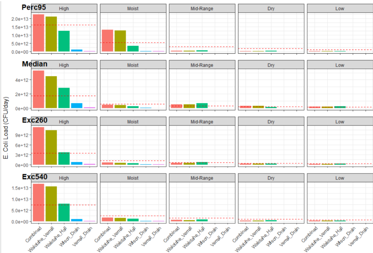
Figure 49 Cumulative E. coli loads at the terminal site (pink bar) and loads from the four water quality sites used in the LDC analysis. Results are split by NPS-FM numeric attribute (top to bottom) and by flow bracket (left to right). The red dashed line represents the swimmability concentration threshold at the terminal reach, i.e., if the combined load exceeds the red line, then the concentration at the terminal reach will be unswimmable.
