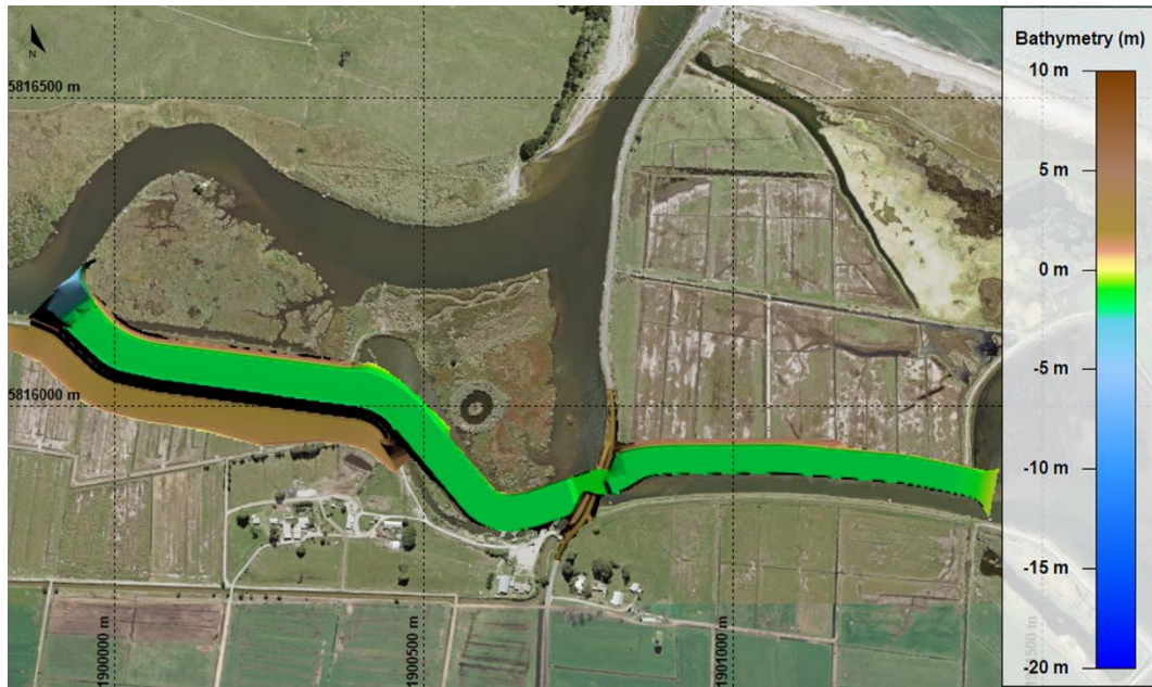
Figure 3-2 Deepened Kaituna re-diversion channel design (Moturiki Vertical Datum).
