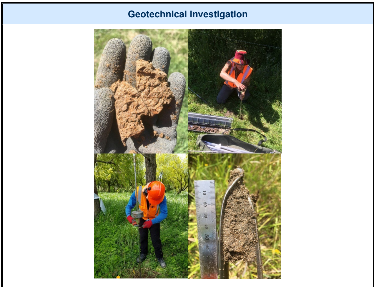
Figure 14 Soil sampling and in situ testing
