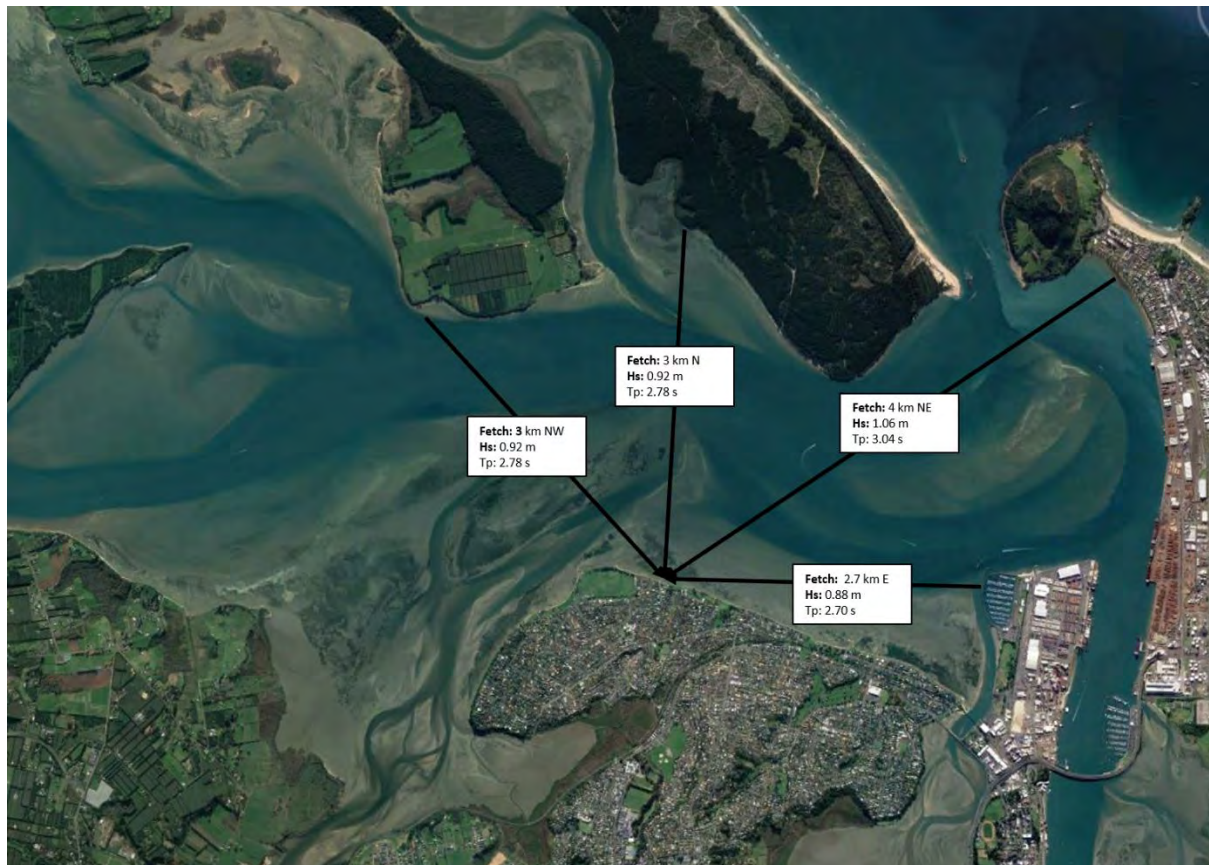
Figure 2-6 Example of fetch distances with corresponding fetch-limited wave heights for the western Otumoetai shoreline. Fetch-limited wave heights based on 23 m/s 1 hour duration wind speeds.
