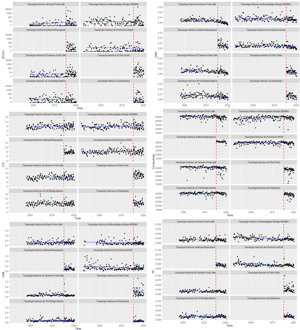
Figure 9.6 Tauranga Harbour compact time-series plots E. coli , dissolved reactive phosphorus, dissolved oxygen (mg/l), conductivity, chlorophyll-a, and total phosphorus. Red dashed line is when the sample time change occurred.
