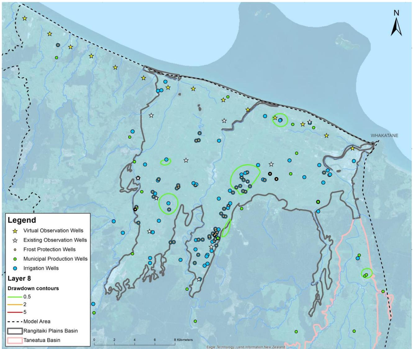
Figure A.8. Drawdown contours for Rangitāiki Plains and lower Taneatua Basin in Layer 8 (layer elevation from about -354 m Moturiki to -317 m Moturiki), stress period 138.
