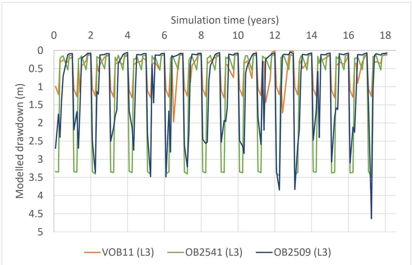
Figure 19. Hydrographs showing modelled drawdown for wells VOB11, 2541, and 2509 (Layer 3)
