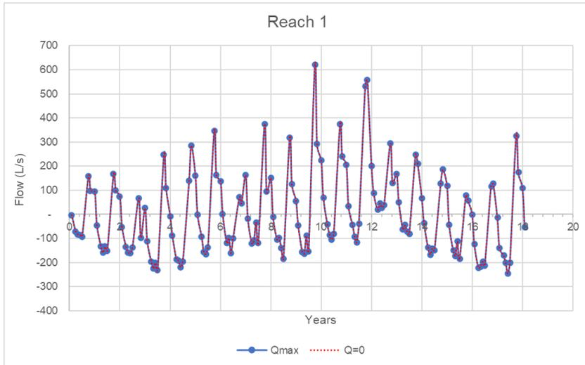
Figure 15. Baseflow for no pumping (Q=0) and pumping at the maximum consented rate (Q=Qmax) for reaches 1.
