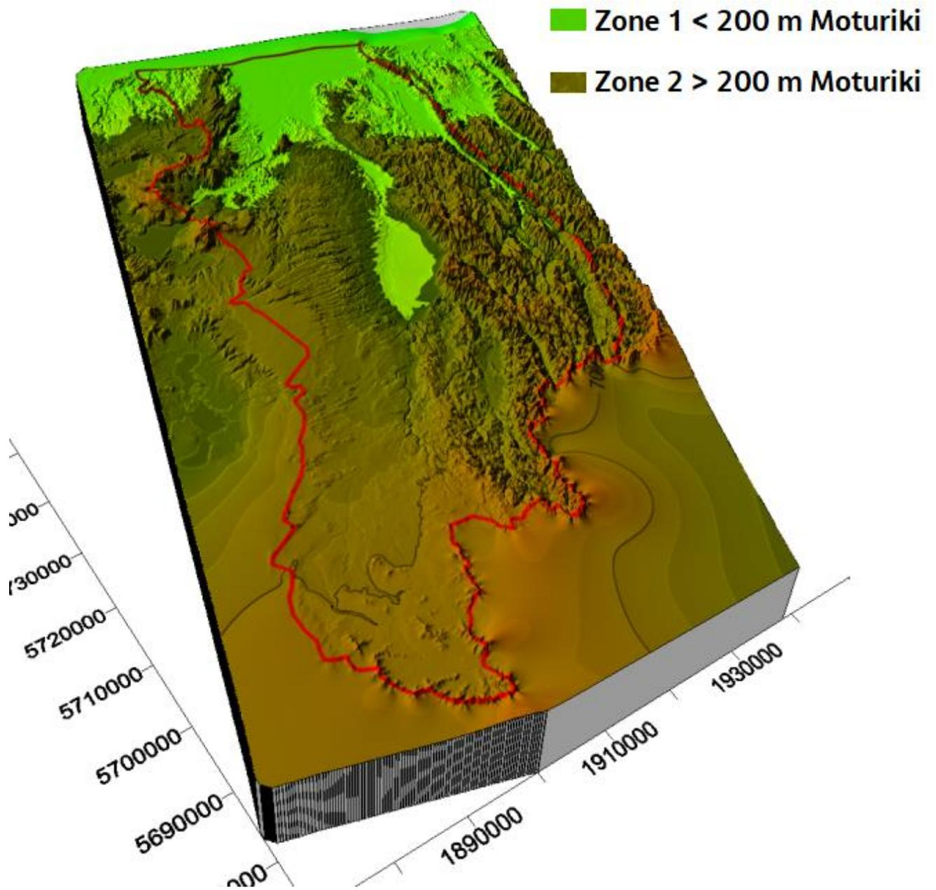
Figure 2. Recharge zones within the RTW model domain
