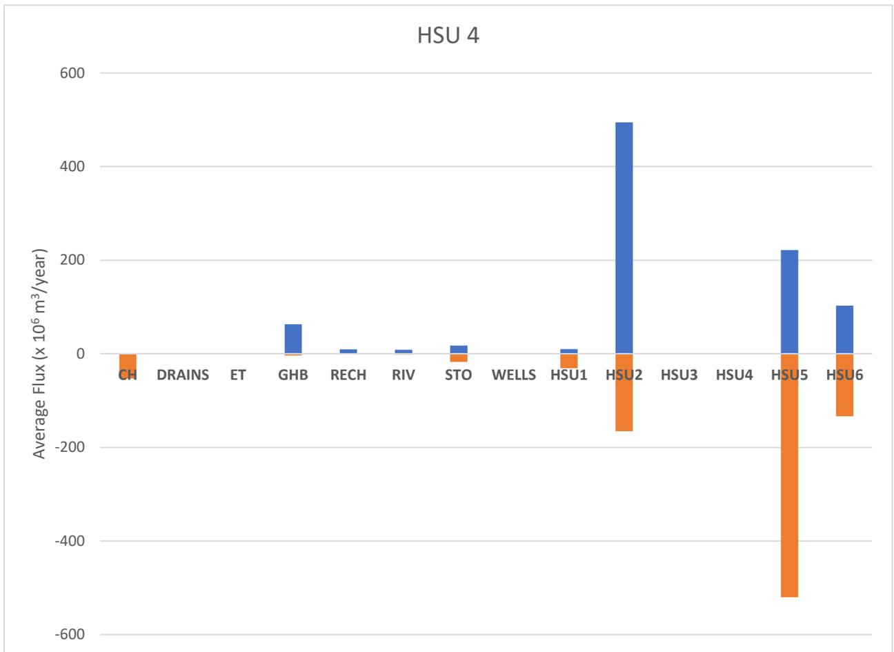
Figure 25. Water balance for HSU 4. Positive flux indicates water flux into the HSU and negative flux indicates water flux out.
