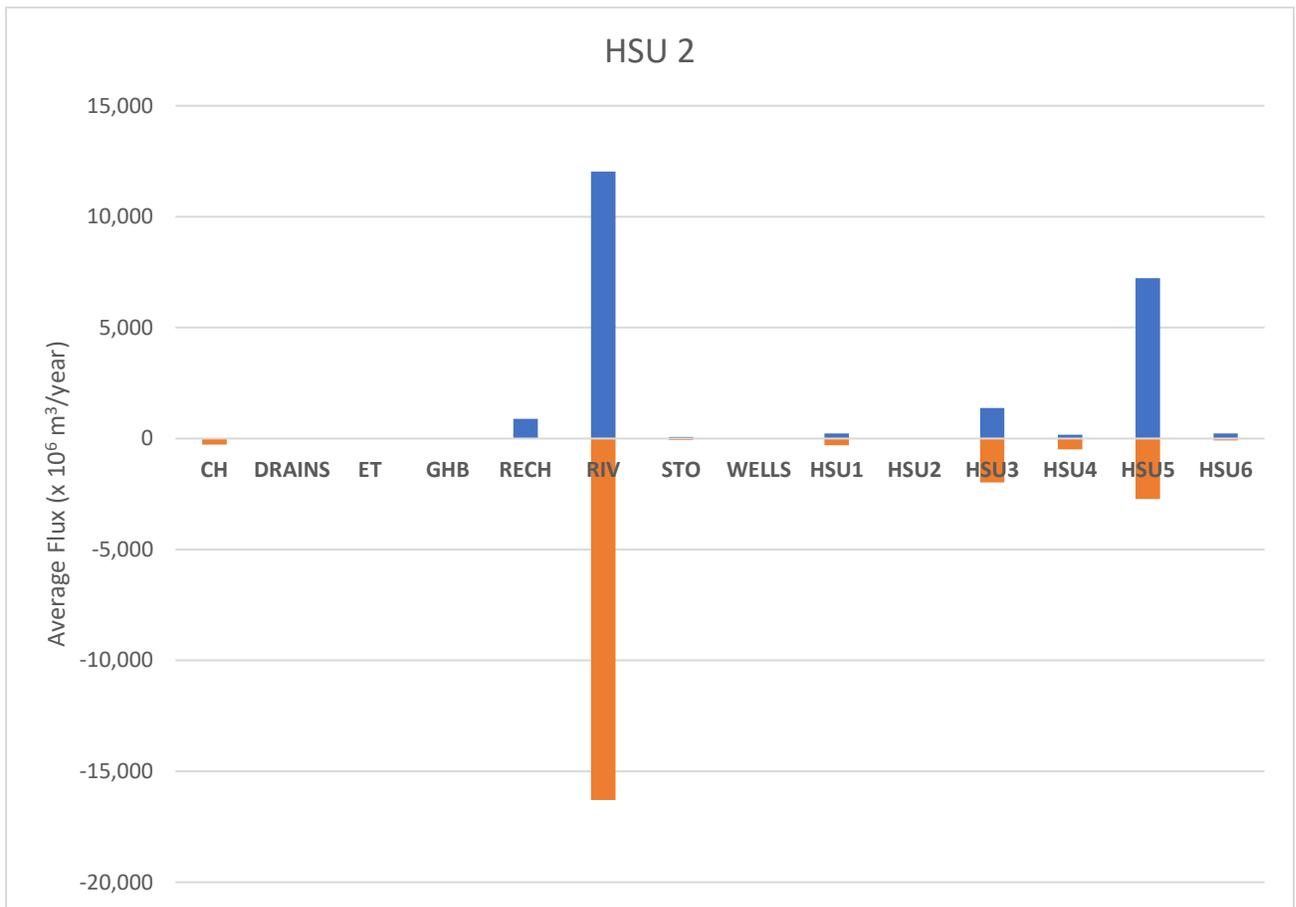
Figure 23. Water balance for HSU 2. Positive flux indicates water flux into the HSU and negative flux indicates water flux out.
