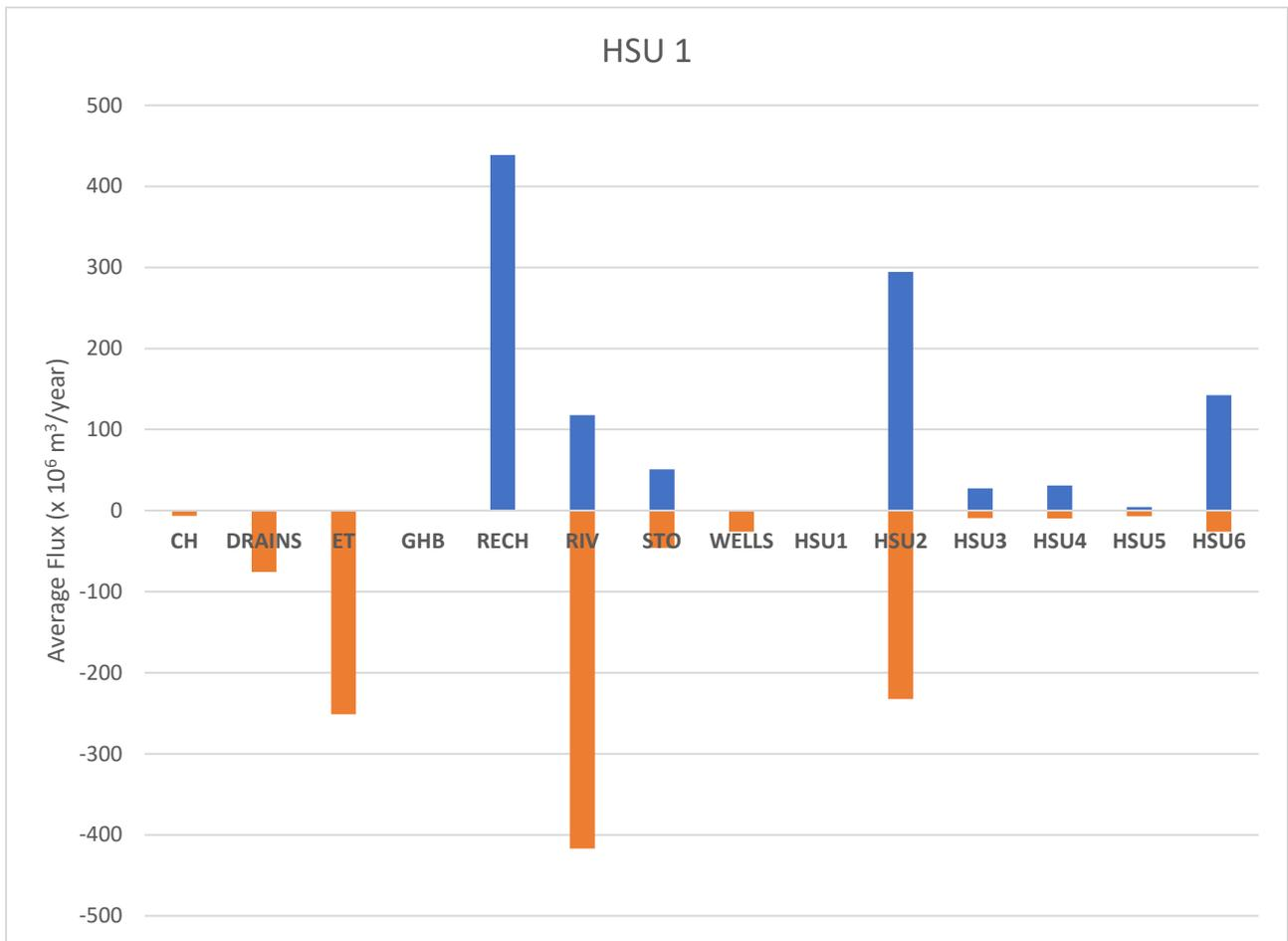
Figure 22. Water balance for HSU 1. Positive flux indicates water flux into the HSU and negative flux indicates water flux out.
