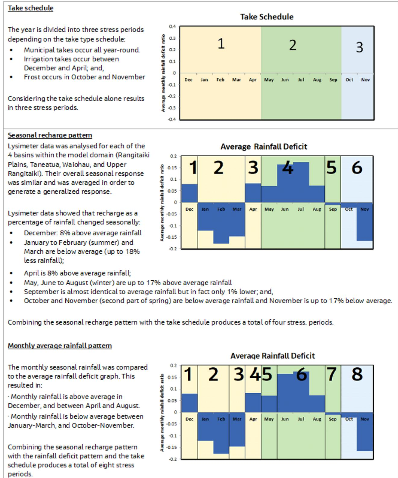
Figure A.1. Derivation of stress periods for the RTW transient model
