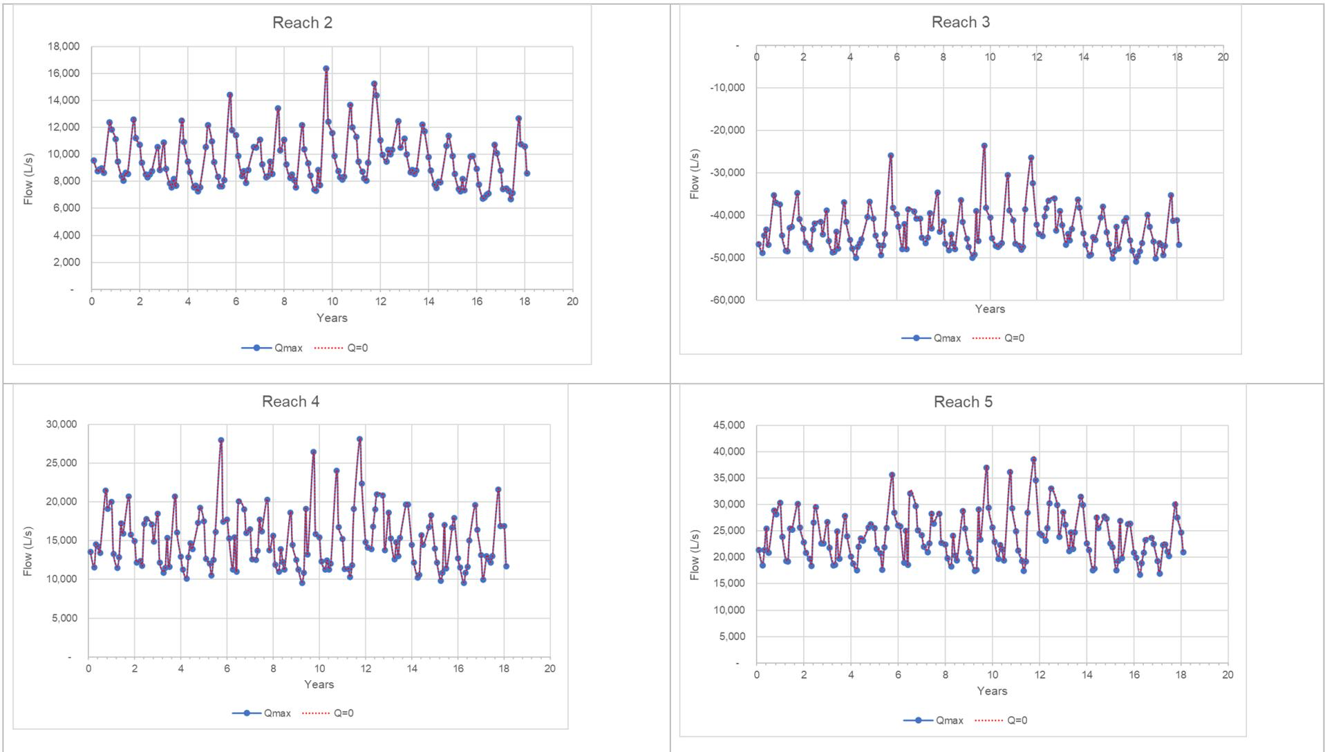
Figure 16. Baseflow for no pumping (Q=0) and pumping at the maximum consented rate (Q=Qmax) for reaches 2 -5
