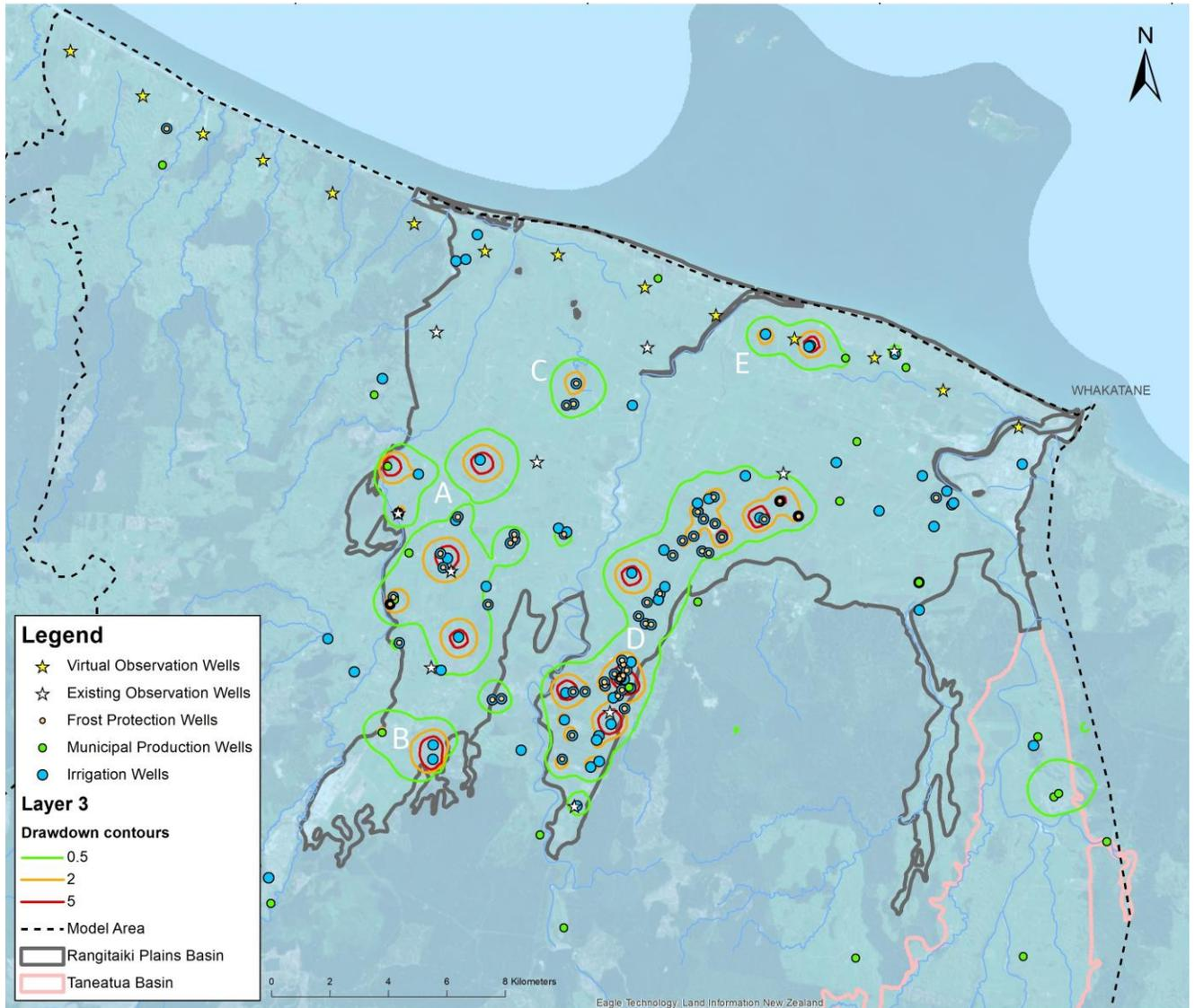
Figure 21. Model predicted drawdown contours (Qmax) for Rangitāiki Plains and lower Taneatua Basin in Layer 3 (layer elevation from about -104 m Moturiki to -67 m Moturiki), stress period 138.
