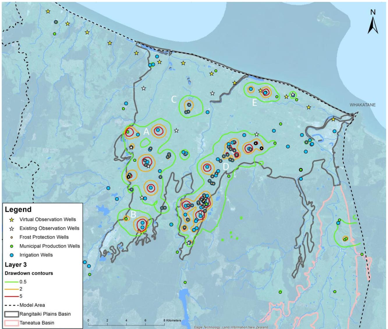
Figure 28. Drawdown contours (1.5 Q<sub>max</sub>) for Rangitāiki Plains and lower Taneatua Basin in Layer 3 (layer elevation from about -104 m Moturiki to -67 m Moturiki), stress period 138.
