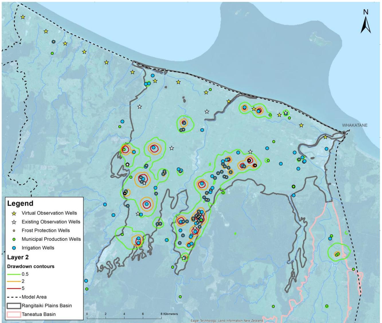
Figure A.3. Drawdown contours for Rangitāiki Plains and lower Taneatua Basin in Layer 2 (layer elevation from about -54 m Moturiki to -17 m Moturiki), stress period 138.
