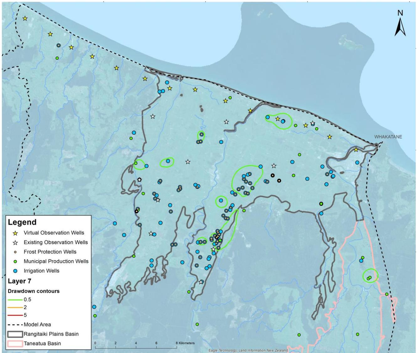
Figure A.7. Drawdown contours for Rangitāiki Plains and lower Taneatua Basin in Layer 7 (layer elevation from about -304 m Moturiki to -267 m Moturiki), stress period 138.
