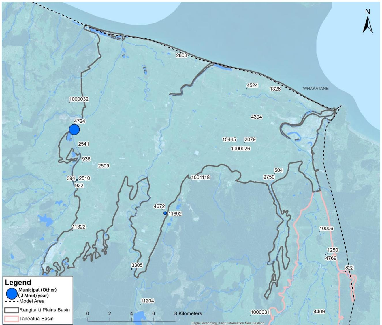
Figure 5. Municipal/Other extraction wells in the Rangitāiki Plains. The symbol size is proportional to their annual groundwater extraction in Mm<sup>3</sup>/year.
