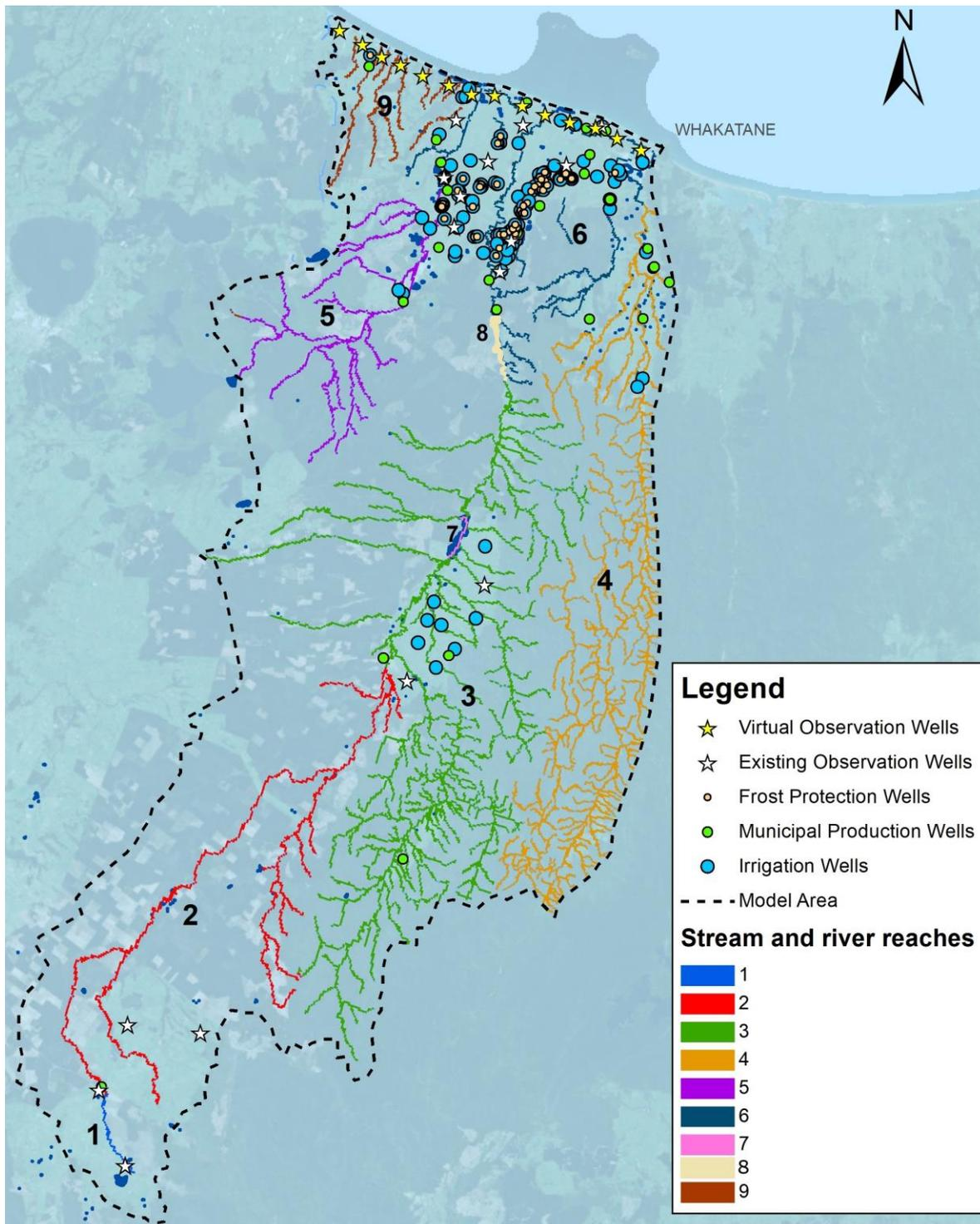
Figure 14. Pumping and observation wells within the model area. This figure also shows the stream and river reaches included in the model domain. Reaches 1 to 6 represent main rivers (Tarawera, Rangitāiki, and Whakatāne rivers) and associated streams. Reach 7 corresponds to the Aniwanuiwa Lake and Reach 8 corresponds to the Matahina Lake at the Rangitāiki River.
