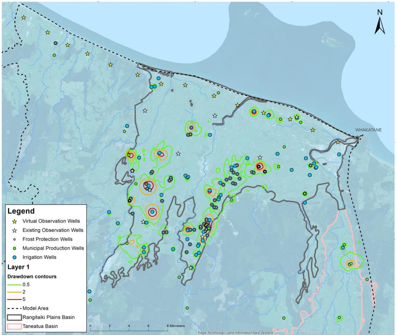
Figure A.2. Drawdown contours for Rangitāiki Plains and lower Taneatua Basin in Layer 1 (layer elevation at natural surface elevation, from about -4 m Moturiki to 32 m Moturiki), stress period 138.
