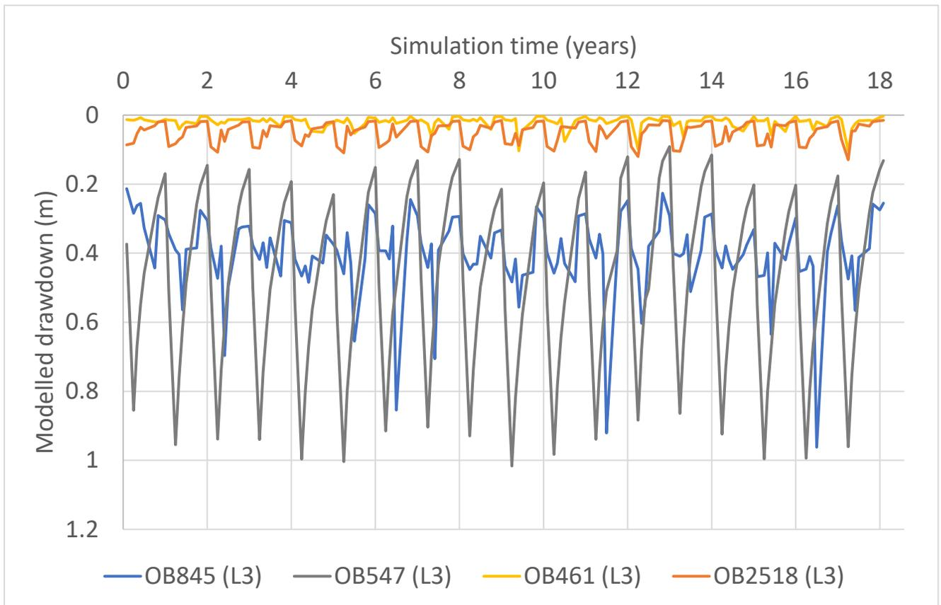
Figure 20. Hydrographs showing modelled drawdown for wells 845, 547, 461, and 2518 (Layer 3)
