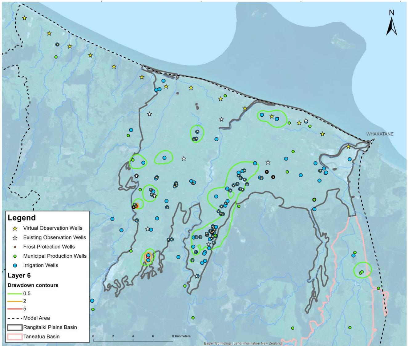
Figure A.6. Drawdown contours for Rangitāiki Plains and lower Taneatua Basin in Layer 6 (layer elevation from about -254 m Moturiki to -217 m Moturiki), stress period 138.
