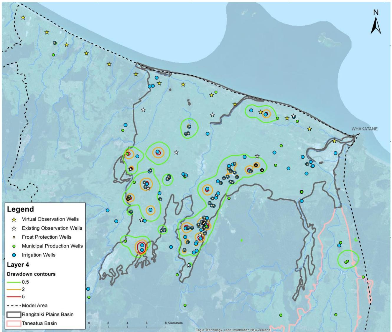
Figure A.4. Drawdown contours for Rangitāiki Plains and lower Taneatua Basin in Layer 4 (layer elevation from about -154 m Moturiki to -117 m Moturiki), stress period 138.
