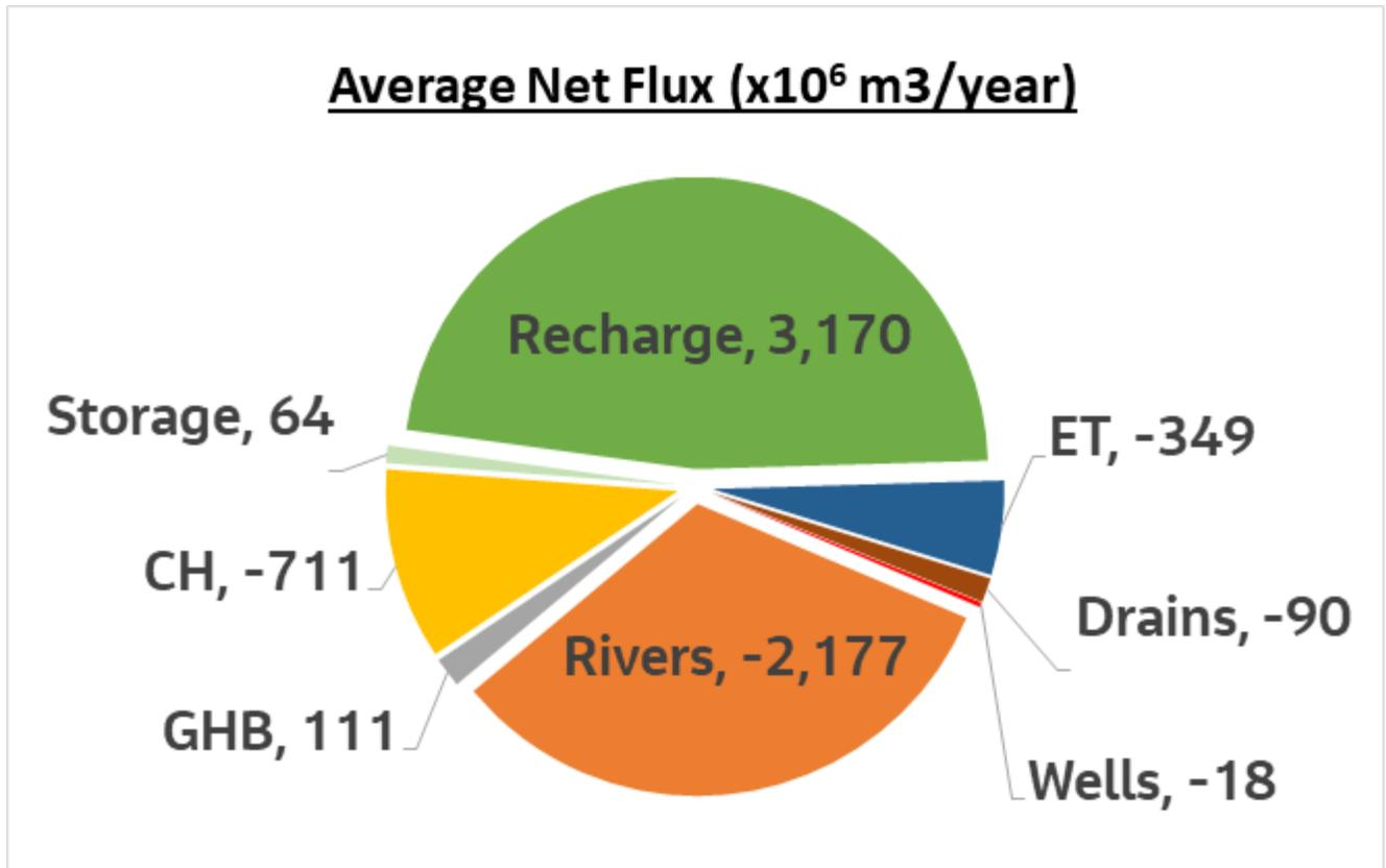
Figure 13. Net average flux for 1985 - 2016 (CH = Constant Head, GHB = General Head Boundary, ET = Evapotranspiration).
