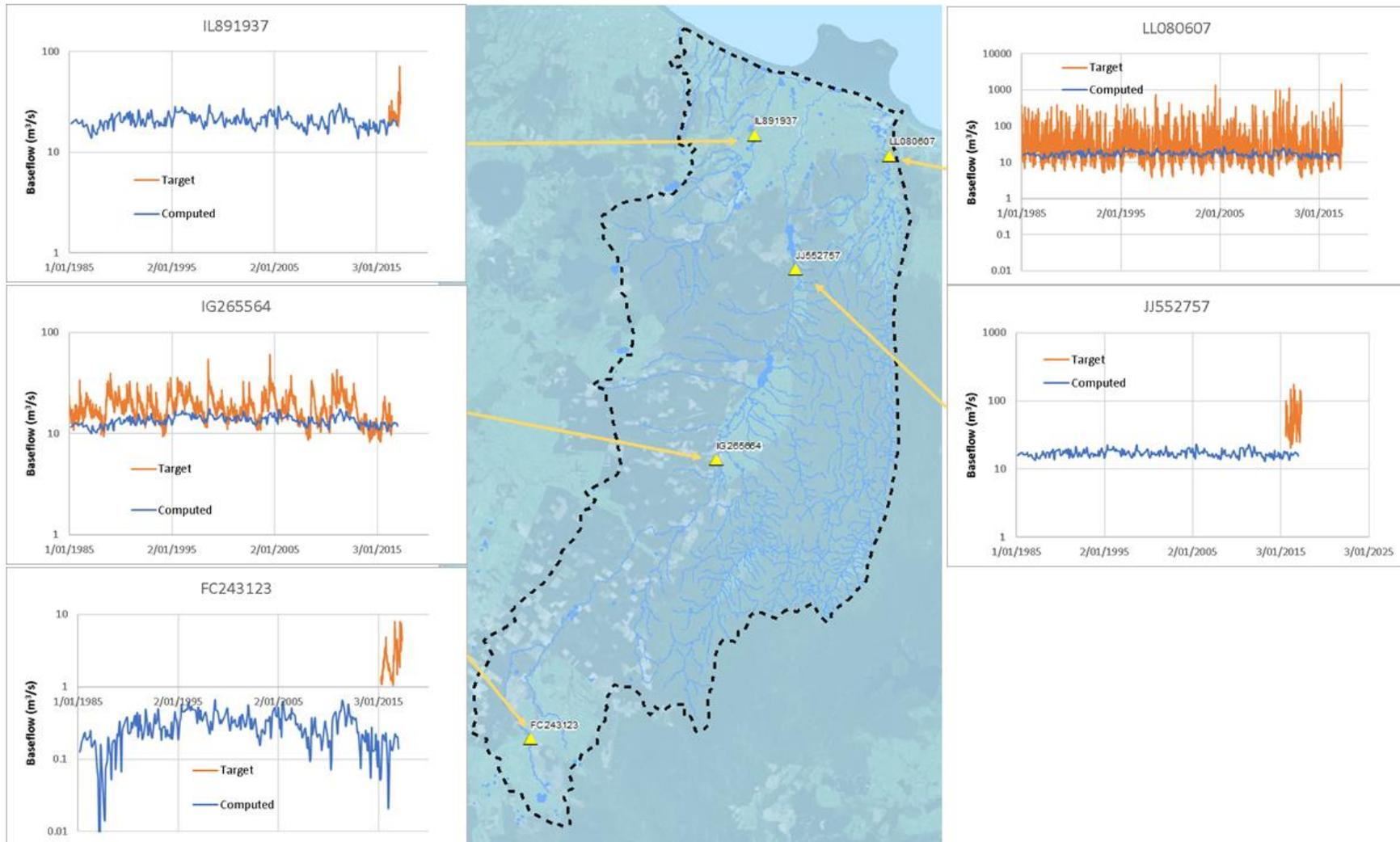
Figure 11. Computed river flux and target river flux comparison
