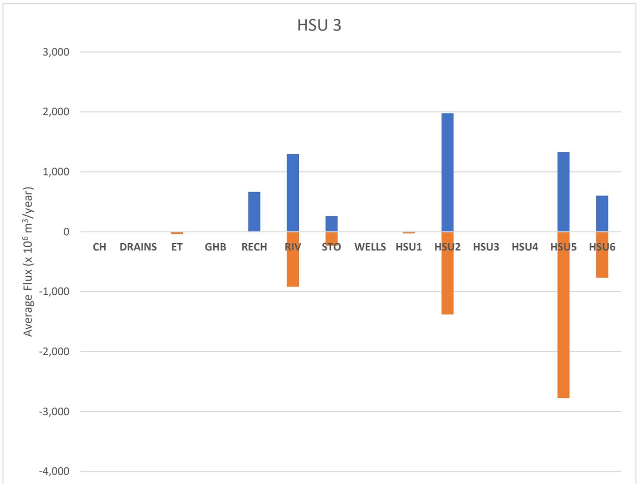
Figure 24. Water balance for HSU 3. Positive flux indicates water flux into the HSU and negative flux indicates water flux out.
