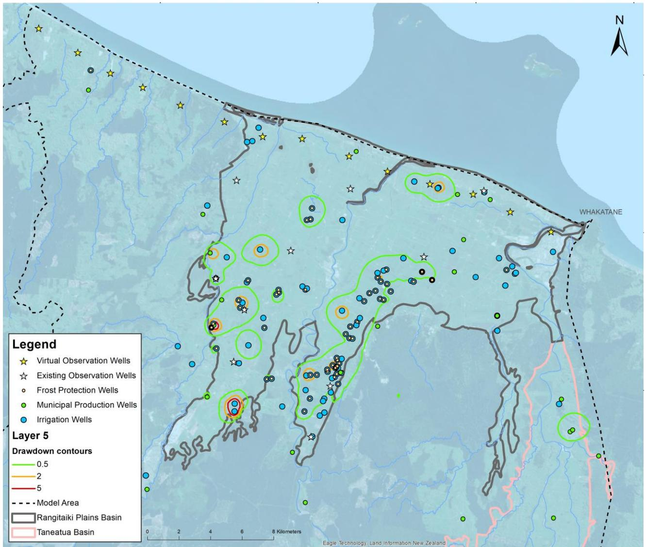
Figure A.5. Drawdown contours for Rangitāiki Plains and lower Taneatua Basin in Layer 5 (layer elevation from about -204 m Moturiki to -167 m Moturiki), stress period 138.
