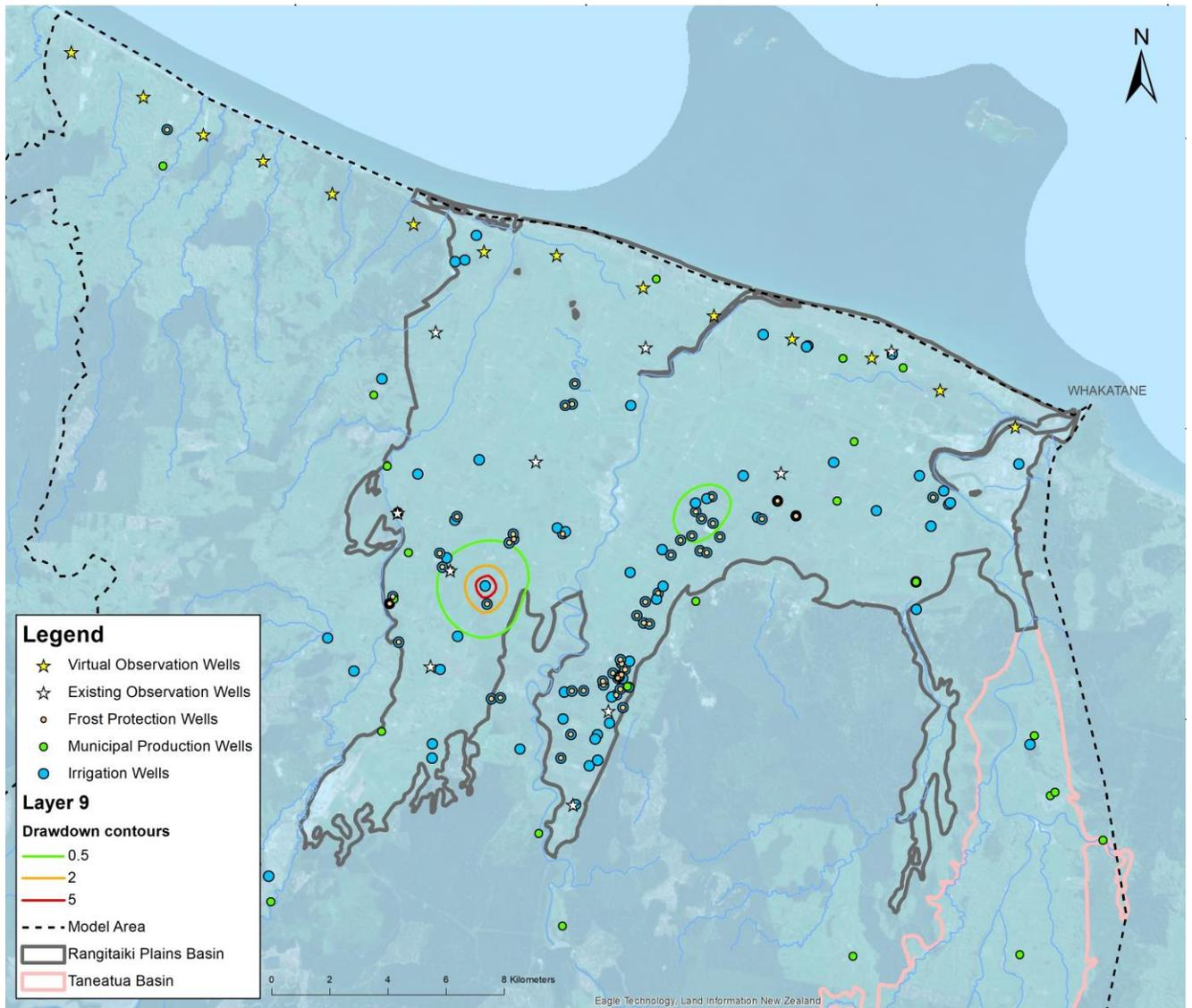
Figure A.9. Drawdown contours for Rangitāiki Plains and lower Taneatua Basin in Layer 9 (layer elevation from about -404 m Moturiki to -367 m Moturiki), stress period 138.
