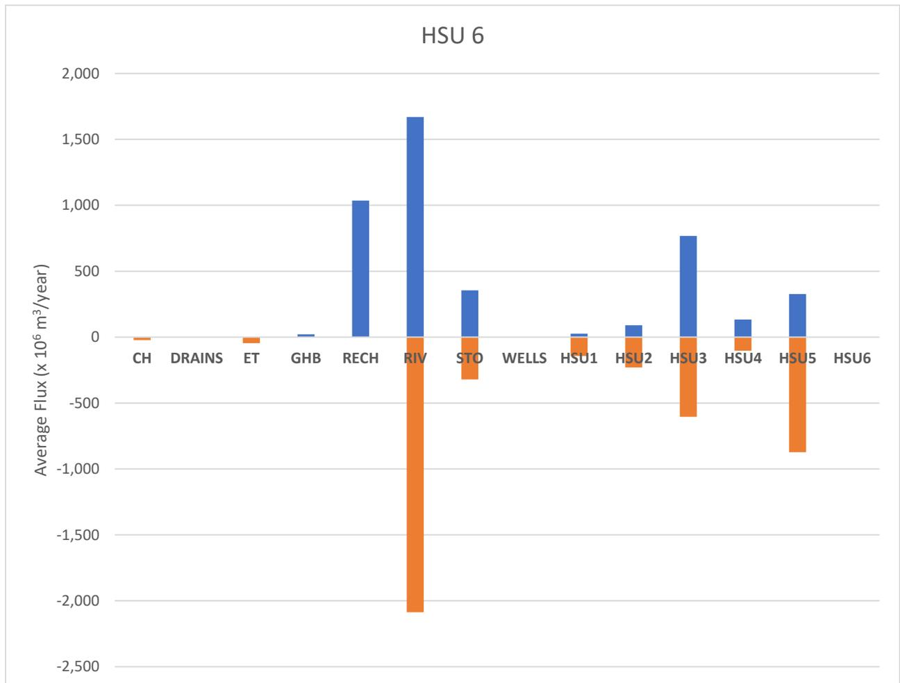
Figure 27. Water balance for HSU 6. Positive flux indicates water flux into the HSU and negative flux indicates water flux out.
