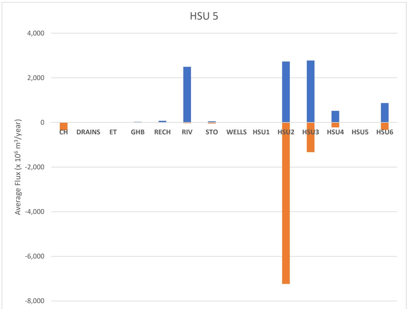
Figure 26. Water balance for HSU 5. Positive flux indicates water flux into the HSU and negative flux indicates water flux out.
