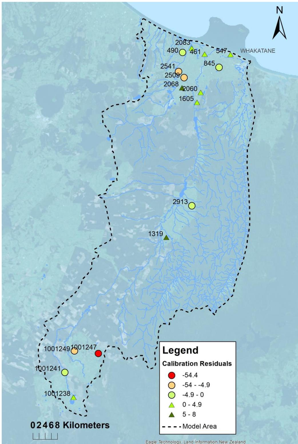
Figure 8. Calibration residual map for Transient calibration (average residuals as Calculated heads minus Observed heads).
