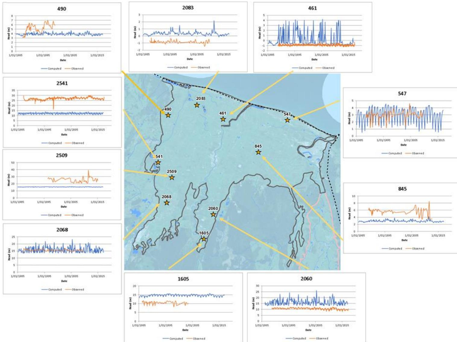
Figure 9. Hydrographs for calibration wells in the Rangitāiki Plains
