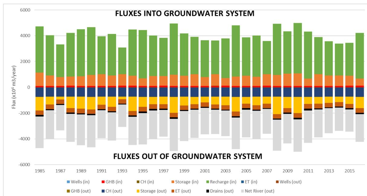
Figure 12. Model mass balance. Fluxes are presented as  $\times 10^6 \text{ m}^3/\text{year}$  on the plot (CH = Constant Head, GHB = General Head Boundary, ET = Evapotranspiration).
