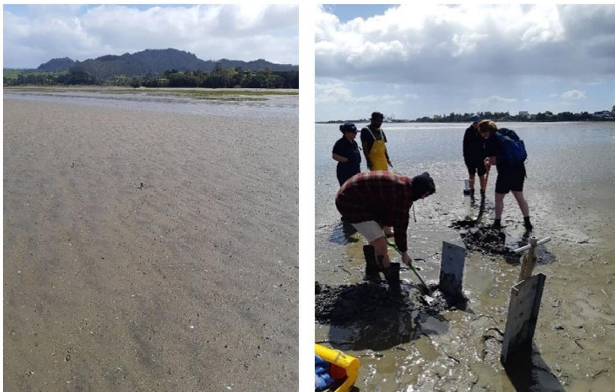
**Figure 2-2: Sediment coring in the study estuaries.** Left: Intertidal sand flat in Tuapiro Estuary (site P54). Right: Perspex-tray trays being used to collect sediment cores in the Waikareao Estuary (site P16) Photos: Greg Olsen.
