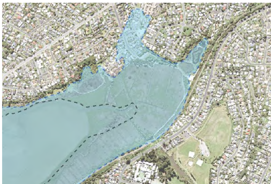
Figure 5-8 Example of how low-lying estuarine shorelines are likely to be translated landward with inundation from future SLR scenarios (black dashed line represents the current MHW, blue shading represents future MHW with 1.6 m SLR).
