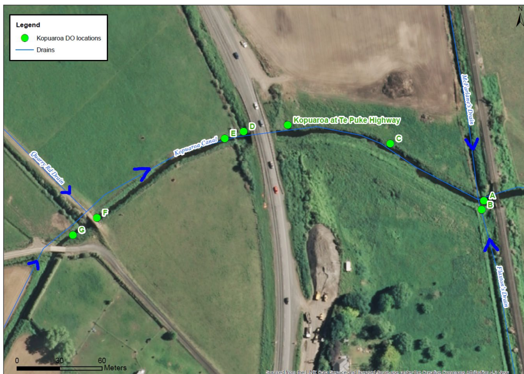
Figure 5.1 Locations for dissolved oxygen investigation in the Kopuaroa Canal, October 2020-March 2021. Location attributes are listed in Appendix C1. Arrows indicate direction of flow.
