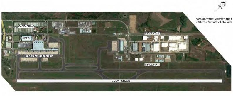
King Shaka International Airport has a 3,7km (1,8-mile) runway, the longest at sea-level in South Africa, and the capacity to accommodate the world's latest and largest new-generation aircraft. It also boasts two rapid exit taxi-ways and the current capacity to handle 23 air-traffic movements every hour.
