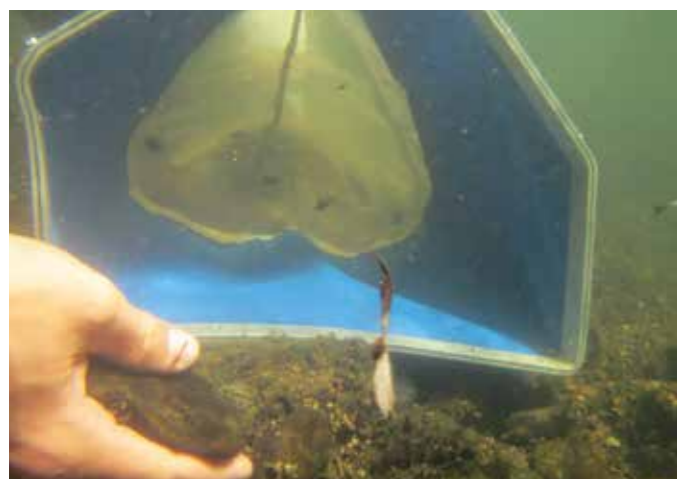
Macroinvertebrates are collected from the streambed by disturbing the streambed immediately above a triangular net, which captures all dislodged material (both invertebrates and organic matter).
