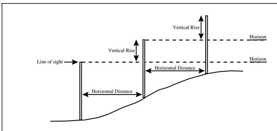
Figure 2.3 Measurement upslope using Emery Pole technique
