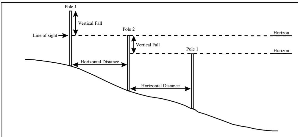
Figure 2.2 Measurement downslope using Emery Pole technique
