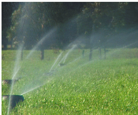
Plate 2. K-line irrigators which may be adapted for use as irrigators of effluent.
