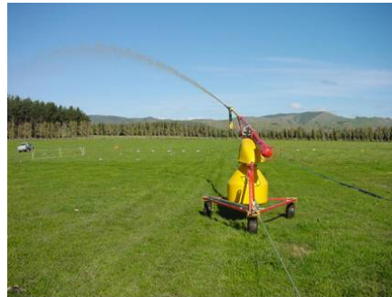
Plate 1. Photographs of the two types of travelling irrigators considered in the simulation. The picture at the top is of a 'Briggs' type standard rotating irrigator (referred to in the text as a 'rotating irrigator'), while the 'Spitfire' oscillating boom travelling irrigator (referred to as an 'oscillating irrigator') is pictured below.
