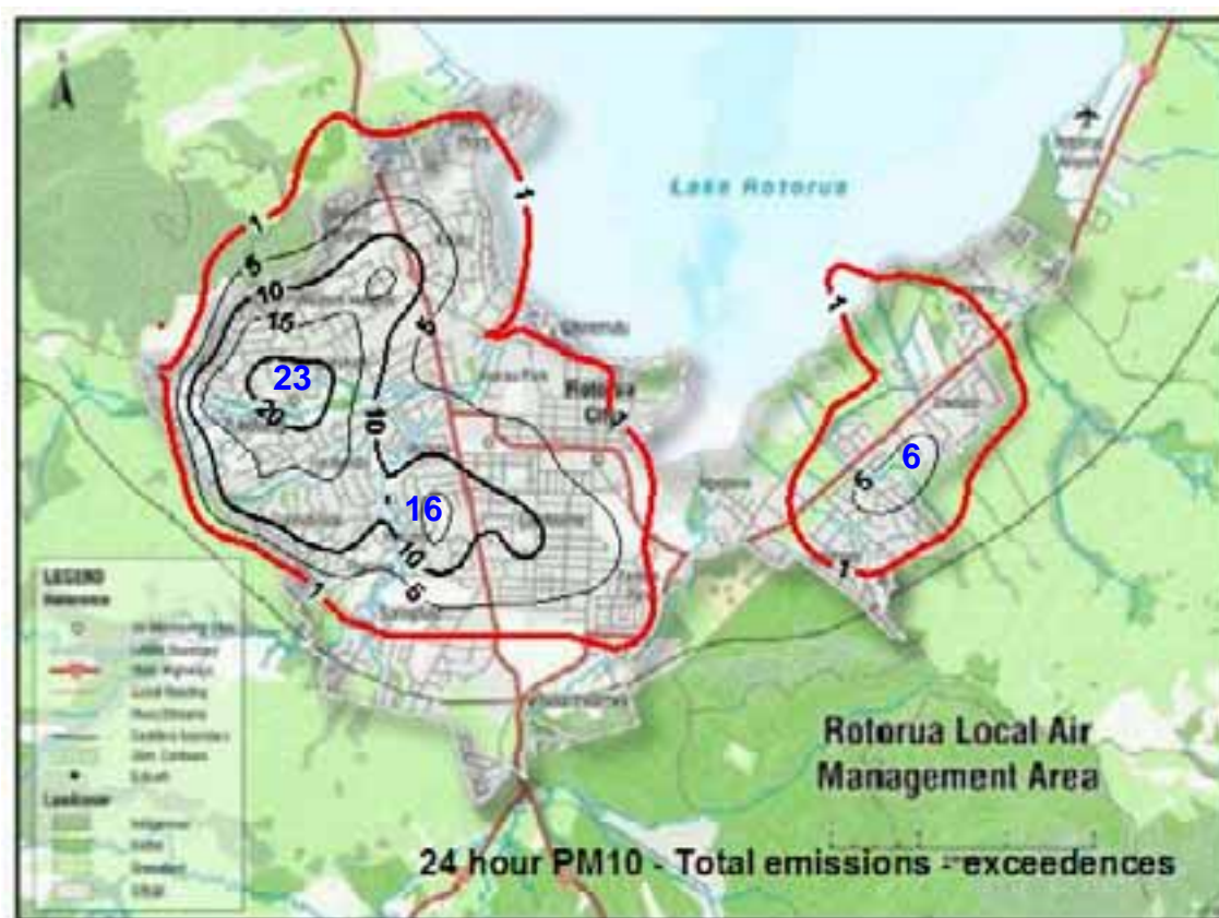
Figure 7.6 The spatial pattern of 24-hour PM 10 exceedences across Rotorua, from total emissions, the worst case results, 2006. (Local peak values also indicated.)
