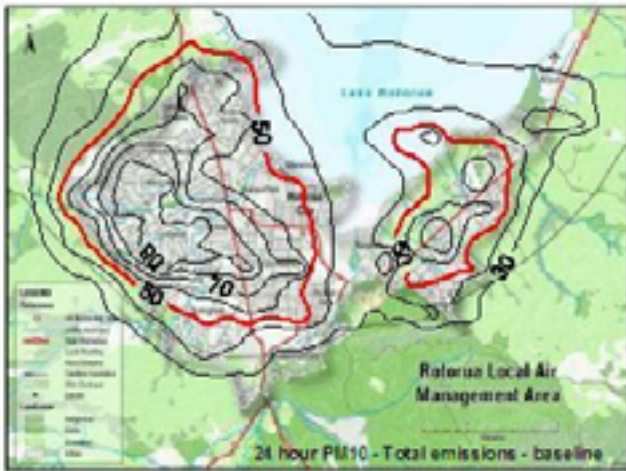
Figure S1. Worst case daily PM_{10} concentrations currently occurring in Rotorua. Areas within the red line exceed the standard of 50 \mu\text{g m}^{-3} .
