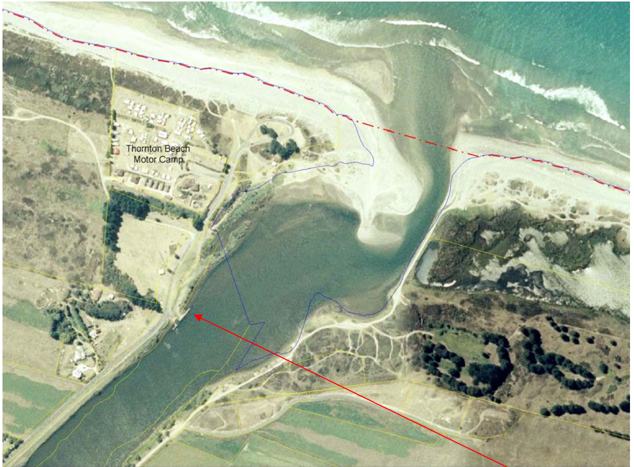
Figure 11 Aerial view of Thornton Bar and the Rangitaiki River Mouth. The Location of Launching Ramps is shown by an Arrow. The Bar formation can be seen at the top of the view
