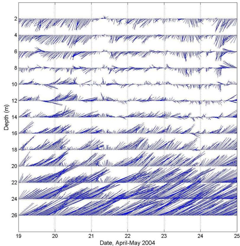
**Figure 3:** Currents measured by ADCP current-meter between 19 and 25 May 2004. Scale: 1 day on the x-axis equals  $0.05 \text{ m s}^{-1}$ . True north corresponds with the vertical axis, depths are relative to the water surface, and “feathers” are in the direction toward
