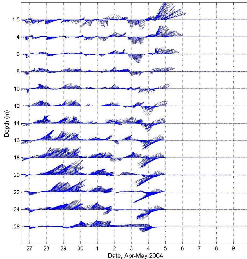
**Figure 2:** Currents predicted by the calibrated model between 26 April and 5 May 2004. Scale: 1 day on the x-axis equals  $0.05 \text{ m s}^{-1}$ . True north corresponds with the vertical axis, depths are relative to the water surface, and “feathers” are in the direction toward which the current is flowing. Feathers are time-averaged over the preceding half-hour and are plotted at half-hour intervals.
