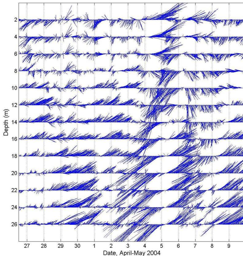
**Figure 1:** Currents measured by ADCP current-meter between 26 April and 10 May 2004. Scale: 1 day on the x-axis equals  $0.05 \text{ m s}^{-1}$ . True north corresponds with the vertical axis, depths are relative to the water surface, and “feathers” are in the direction toward which the current is flowing. Currents were recorded every 5 minutes, but are plotted at half-hour intervals after smoothing with a half-hour running-average.
