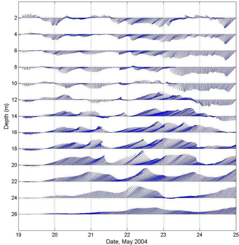
**Figure 4:** Currents predicted by the calibrated model between 19 and 25 May 2004. Scale: 1 day on the x-axis equals  $0.05 \text{ m s}^{-1}$ . True north corresponds with the vertical axis, depths are relative to the water surface, and “feathers” are in the direction toward which the current is flowing. Feathers are time-averaged over the preceding half-hour and are plotted at half-hour intervals.
