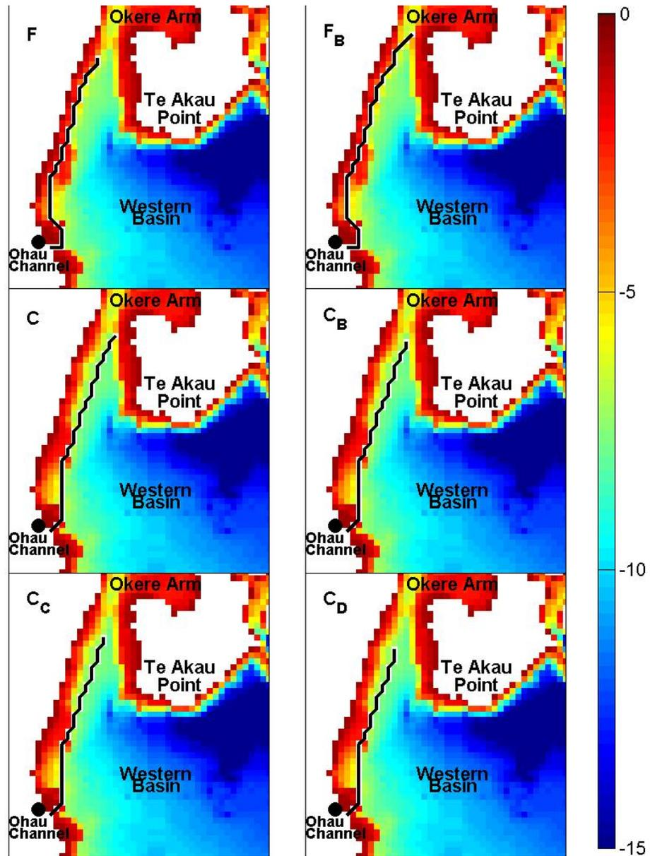
**Figure 5:** Depth-shaded bathymetry maps showing simulated wall locations; walls are variations on Options C and F (Stephens, 2004, Table 1, Figure 23). Option F<sub>B</sub> has been extended from the original, whereas options C<sub>B</sub>, C<sub>C</sub> and C<sub>D</sub> become progressively shorter than the original. Dry areas are shaded white.
