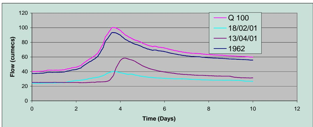
Figure 4 Hydrographs Used in the Tarawera River Capacity Model
