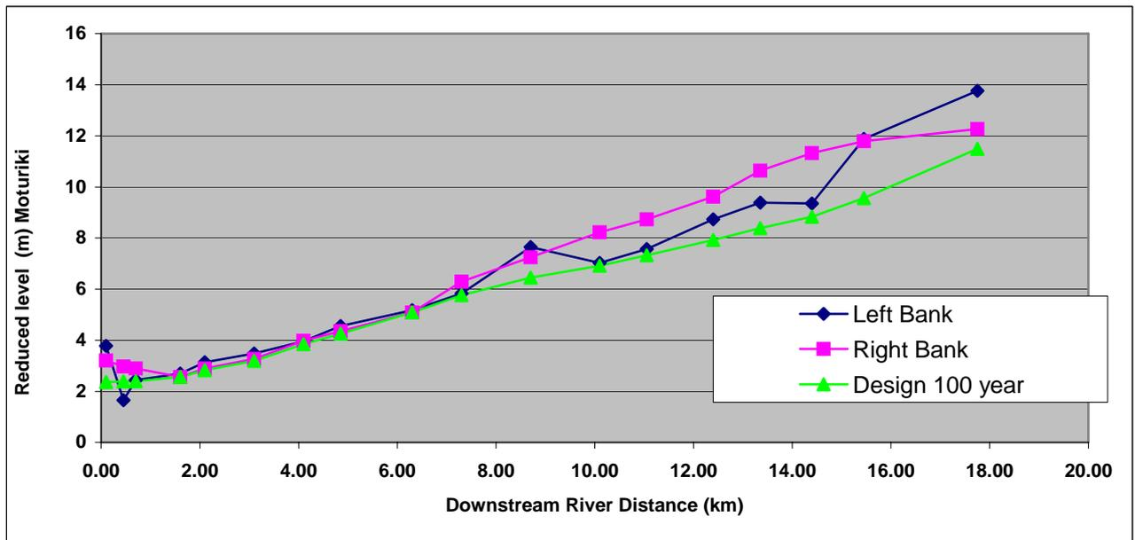
Figure 10 Tarawera River Stopbanks and Combined 1% AEP Water Levels
