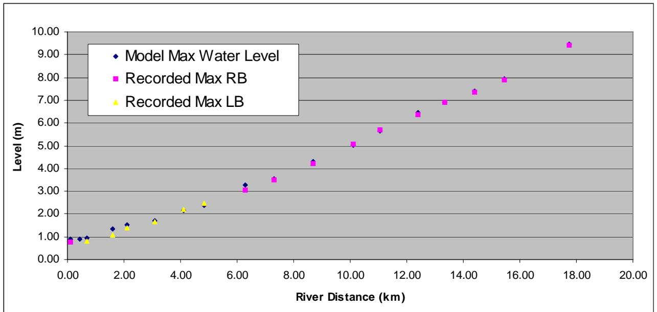
Figure 6 Graph Showing Calibration of Recorded and Modelled Flood Levels
