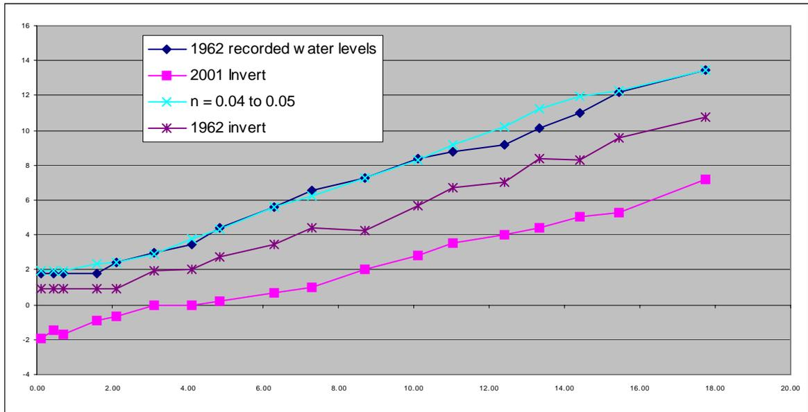
Figure 9 Plot Showing Calibration to the 1962 Recorded Flood Levels
