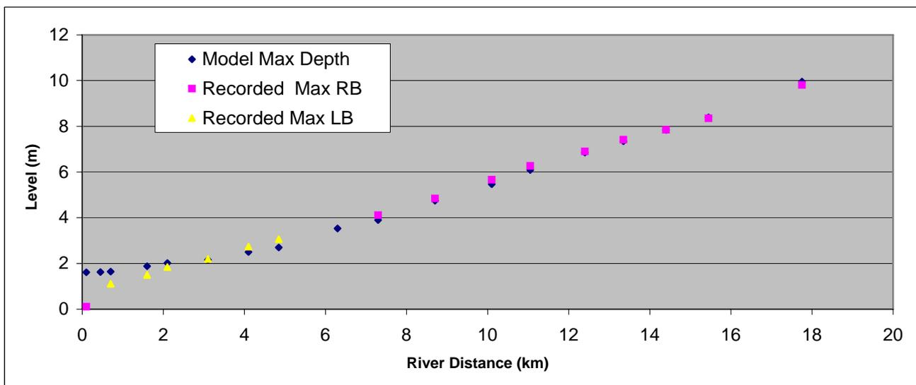
Figure 7 Graph showing verification of recorded and modelled flood levels
