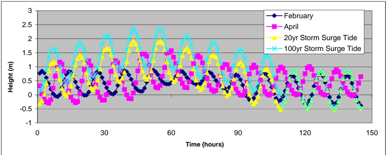
Figure 5 Tides Used in the Tarawera River Capacity Model
