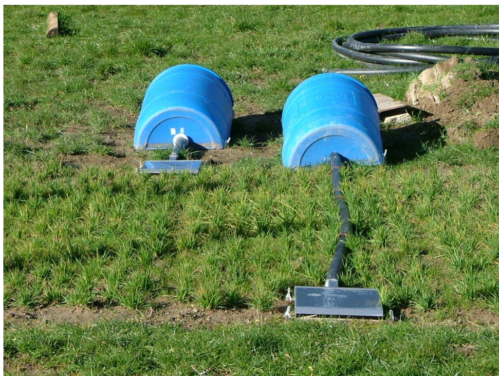
Figure 5: Inflow (foreground) and outflow collectors on the Phalaris plot at Rerewhakaaitu (Lucy McKergow, 21 July 2007).
