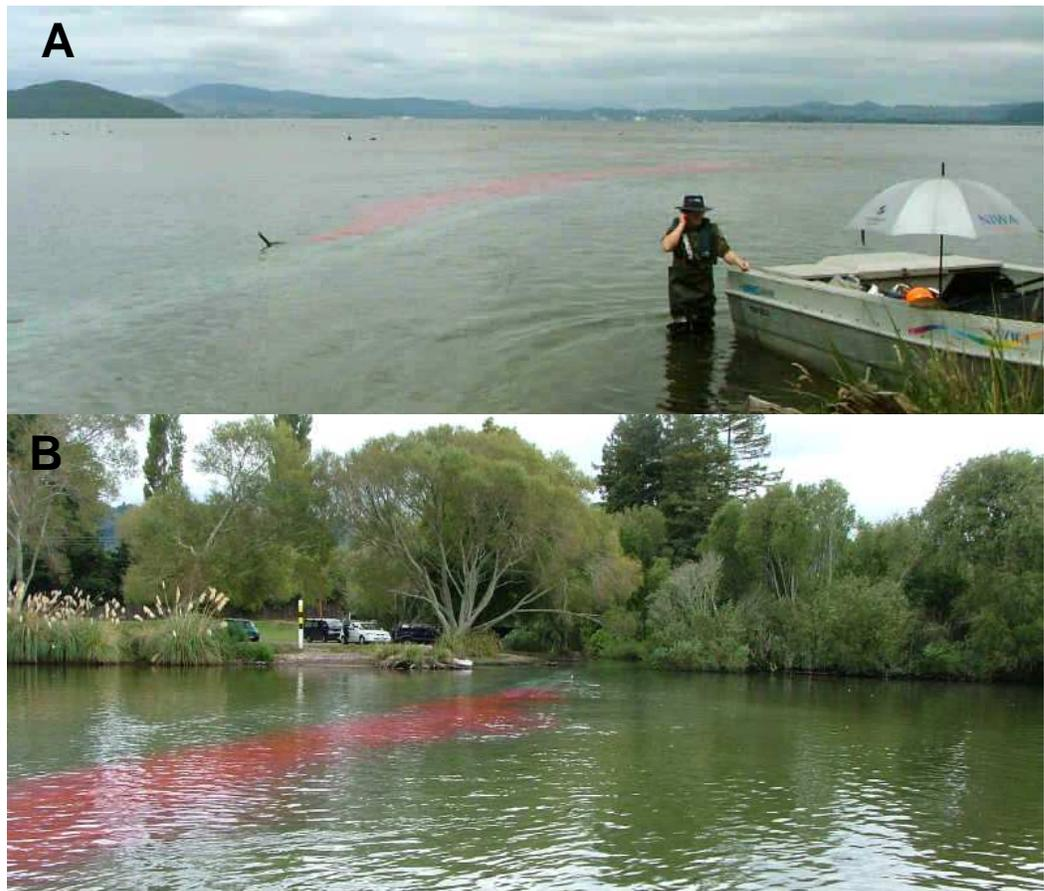
**Figure 2:** Dye injection showing the dye movement as a thin ribbon from the injection point A) looking from shore and B) looking back towards the shore.
