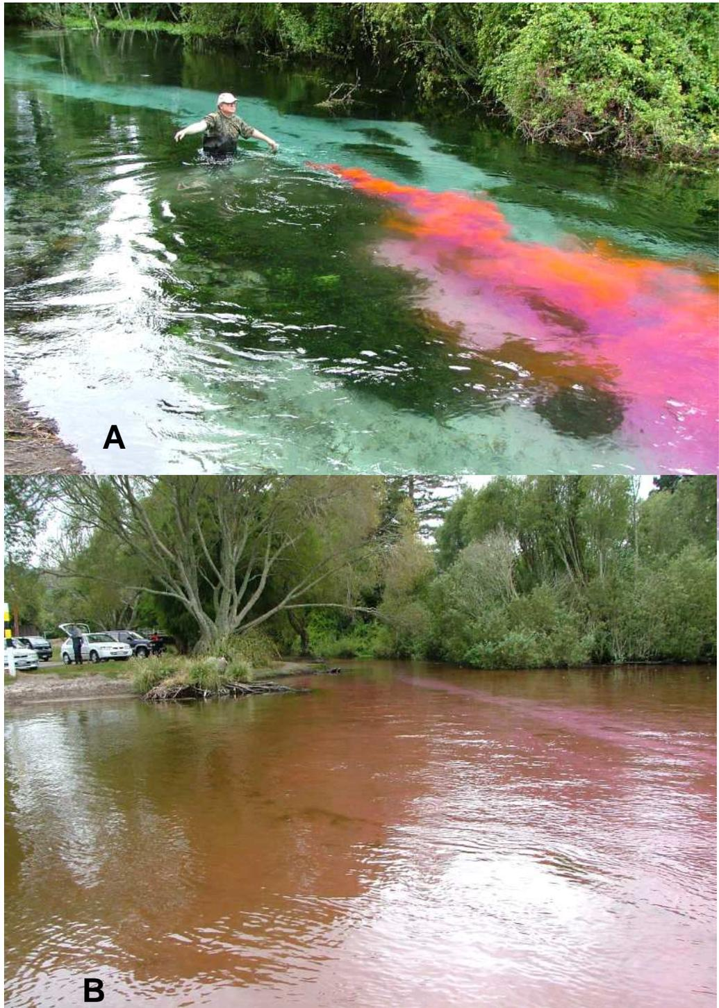
**Figure 1:** A) Dye injection in the Hamurana Stream, B) Dispersion and pooling of the dye in the cold water trout refuge zone on the shallow shelf.
