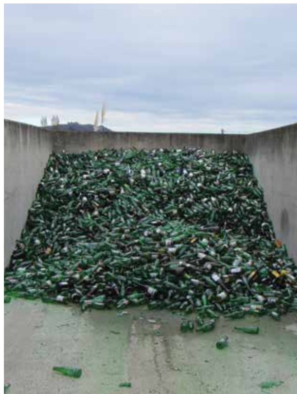
Glass separation for recycling
