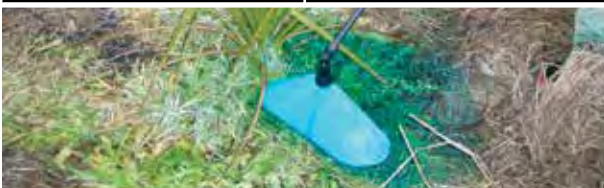
Spray cone on nozzle to avoid spray drift. Blue dye is used to show where you've sprayed
