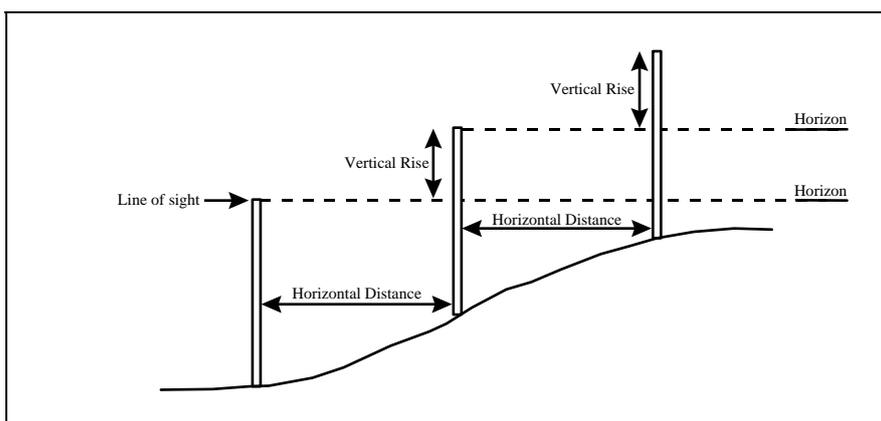
Figure 10 Measurement upslope using Emery Pole technique
