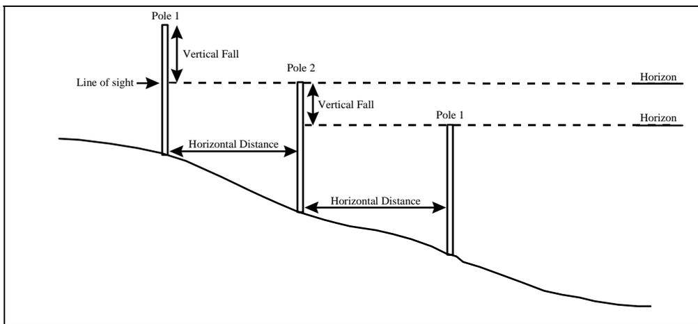
Figure 9 Measurement downslope using Emery Pole technique
