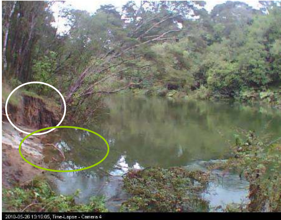
Figure 3-53: Site 4 after flood waters had receded on 26/5/10. Circed areas show site of soil loss (white) and vegetation removal (green) in comparison with photo taken on 24/5/10.
