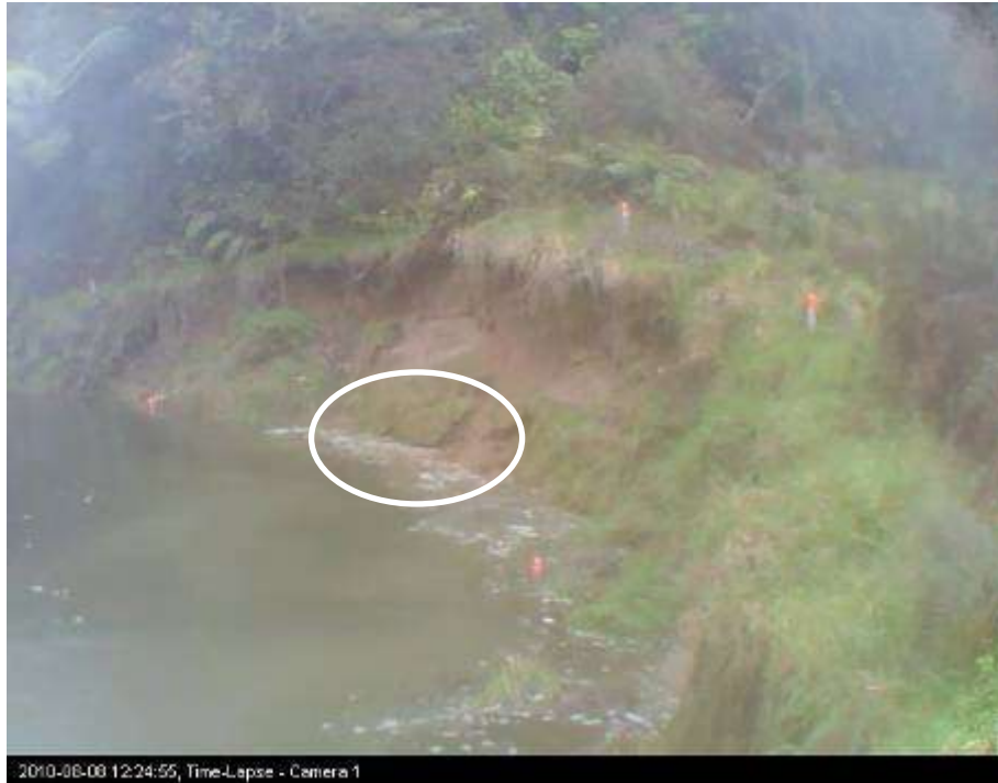
Figure 3-27:Active erosion at waters edge at Site 1 on 8/8/10 12:25. 5 mins after the previous photo. Note the peg in the circled area has disappeared.
