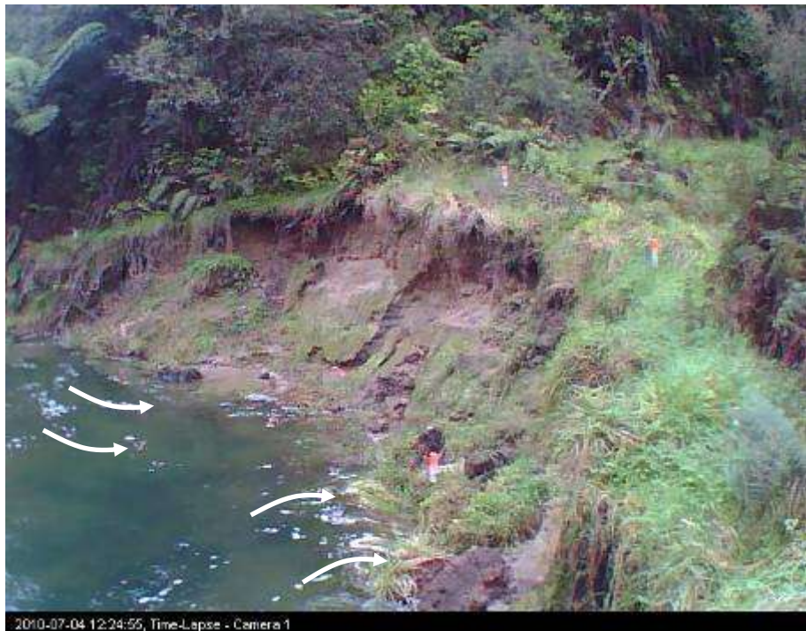
Figure 3-23:Site 1 on 4/7/10 at 12:25, just as a small wave is hitting the bank. It is assumed that this wave has been generated by a jet boat.
