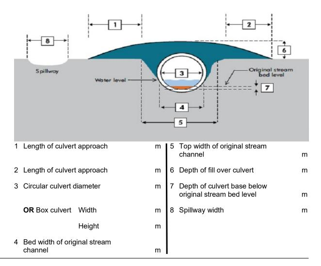
5 **Other in-stream works** (e.g. bank stabilisation, erosion protection features, retaining works, fords, pipes).
