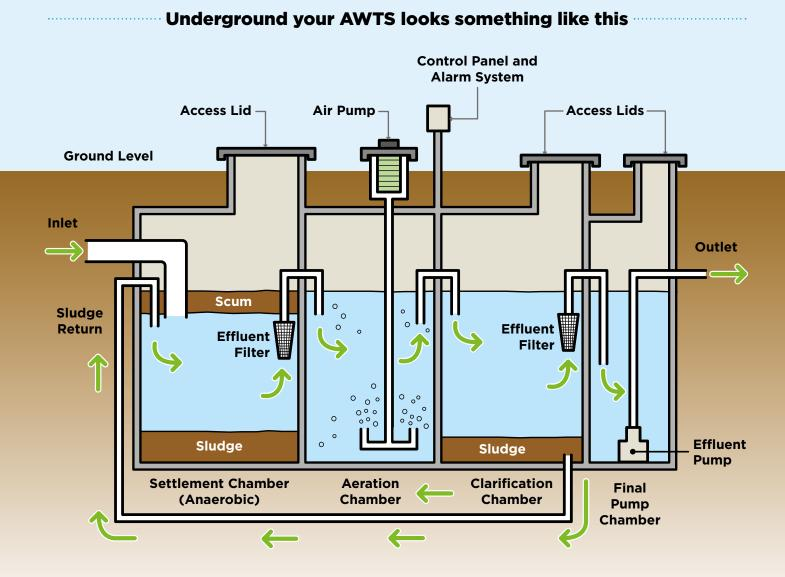
To effectively process wastewater, and to avoid odours and 'ponding', your AWTS needs regular maintenance by a trained technician every six months.
