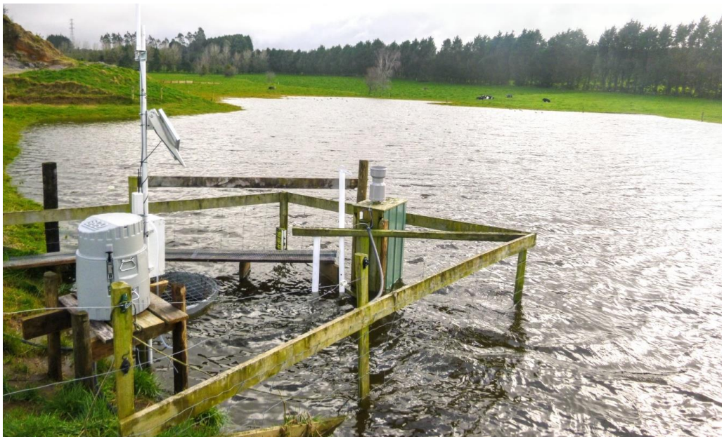
Figure 2.1: Photo of a pond formed on pasture by a detainment bund impeding the flow of surface runoff generated during a storm event. The fencing protects sampling equipment from livestock.
