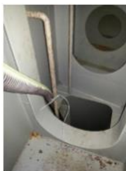
Nova-flow pipe installed allowing pallet fumigation
