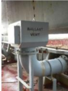
Large purging valve, only found at hold 3.
