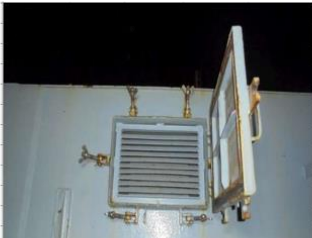
Natural vent with grill on & door open.
