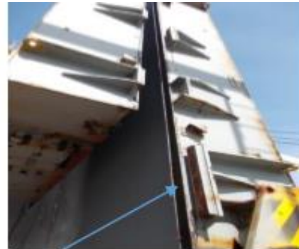
Rubber seals must be in good condition
