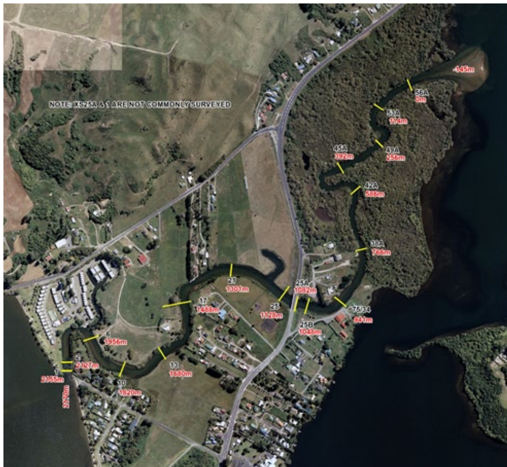
Figure 16 Ohau Channel cross section locations.
