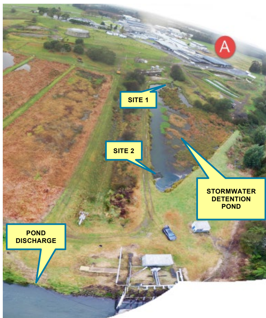
Figure 1-1: AFFCO Rangiora Plant stormwater detention pond showing discharge point and sampling locations
