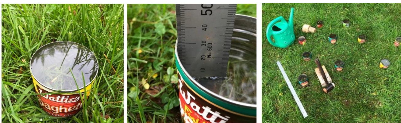
Figure 14 JP bean can single ring infiltrometer (best used in sample plots of 10 cans).
