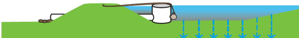
Figure 5E Sediment settling and pond water infiltration continues for up to three days.
