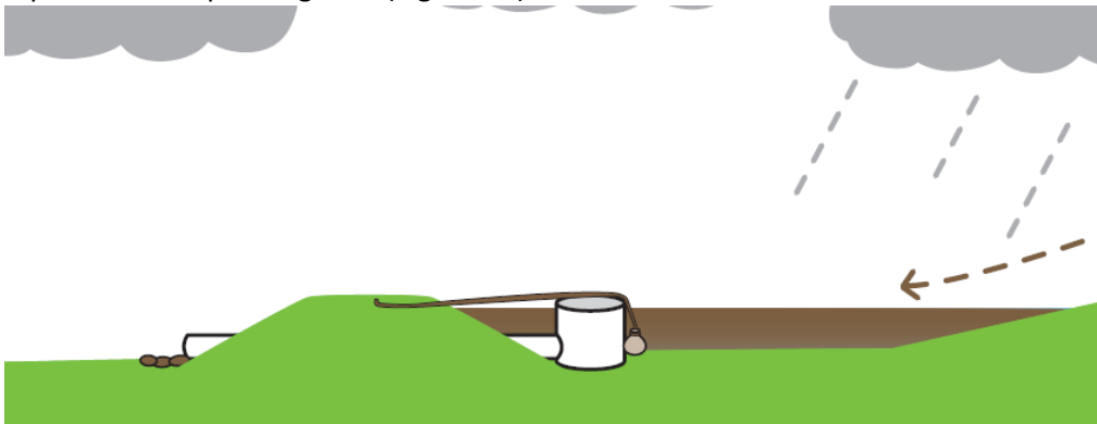
Figure 5B DBs capture dirty storm water run-off during high intensity rainstorm events.
