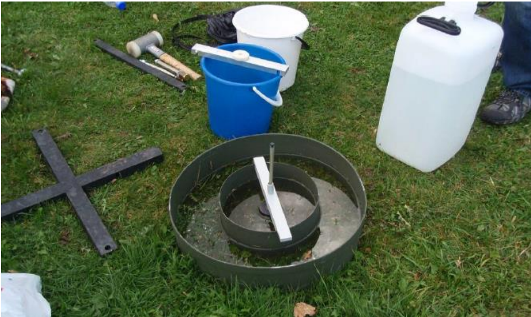
Figure 12 Measuring the infiltration rate of pasture soil with a double ring infiltrometer.
