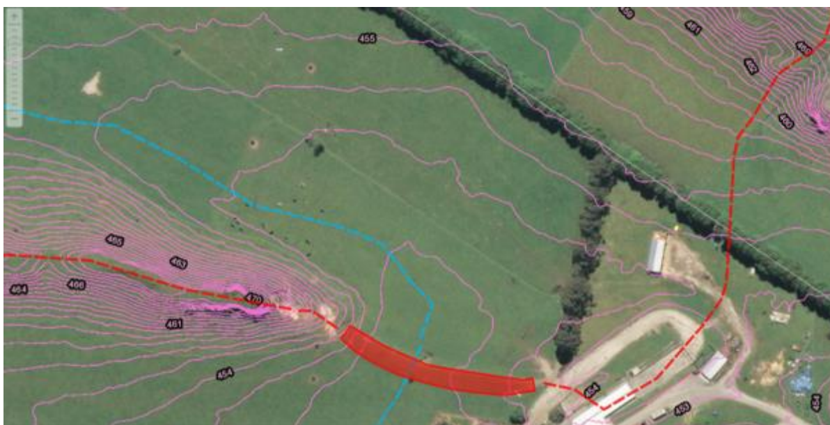
Figure 15 LiDAR data enables 1 m contour detail. The red polygon is an example DB 'mock-up'.
