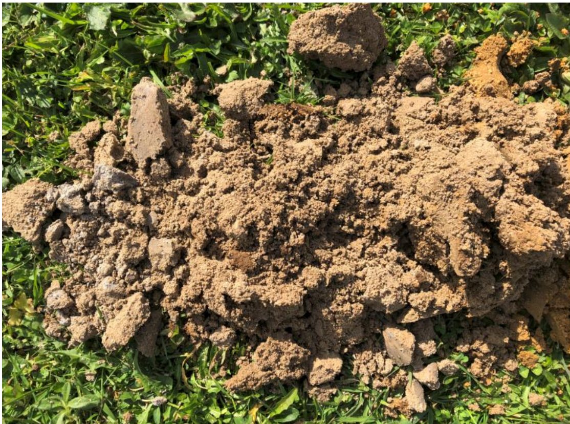
Close up of Weathered Ignimbrite with fragments of unweathered rock (light grey-white) at left
