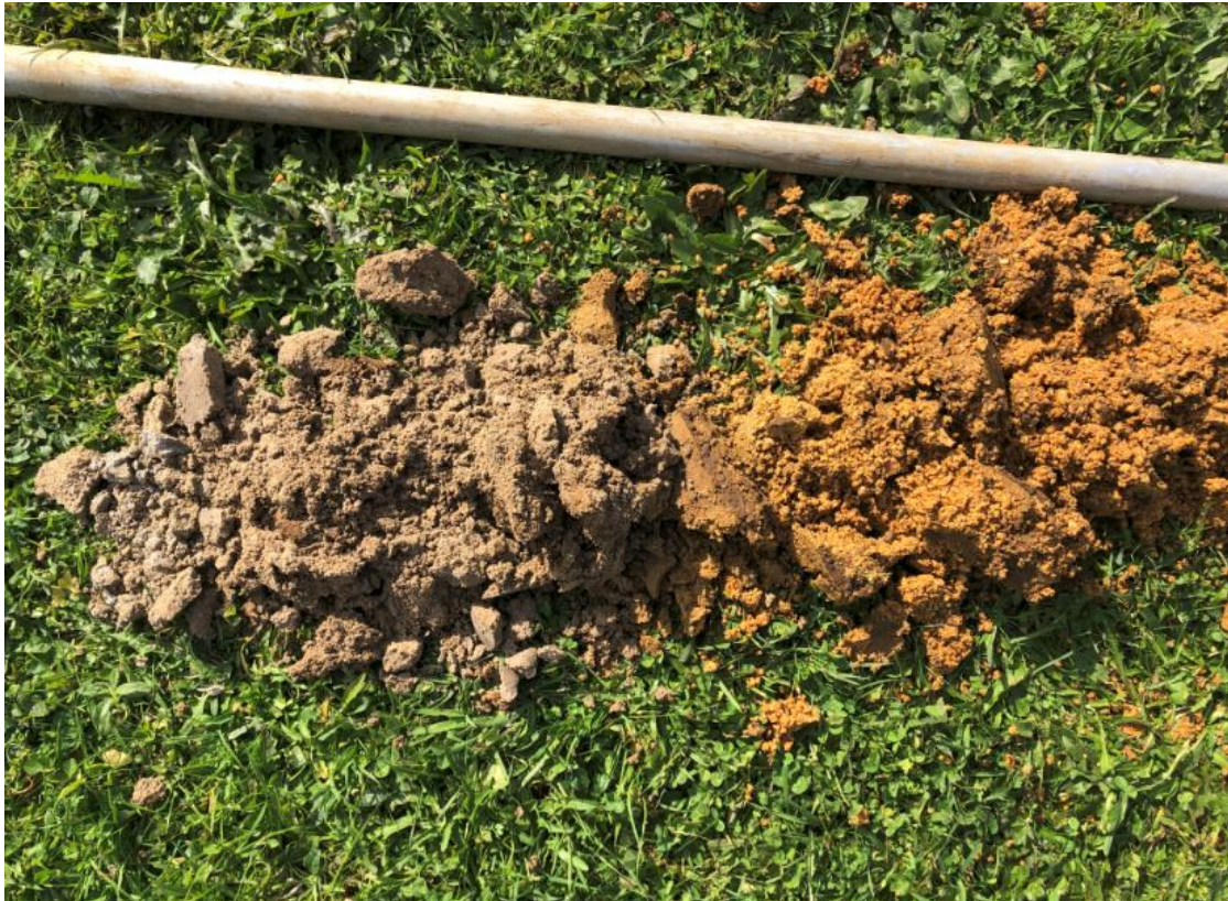
Transition between Gravelly Silt Ash and Weathered Ignimbrite (Silt, light grey, stiff, moist)
